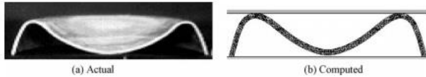
Figure 15. Comparison of actual and FEA predicted failure of spherical shell
