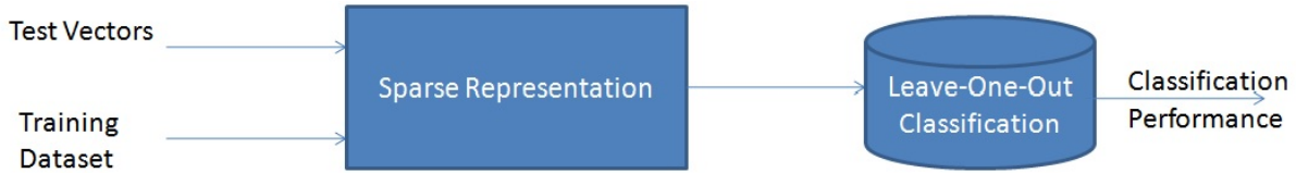
Figure 4.2: The block diagram explaining the procedure while using sparse representation
