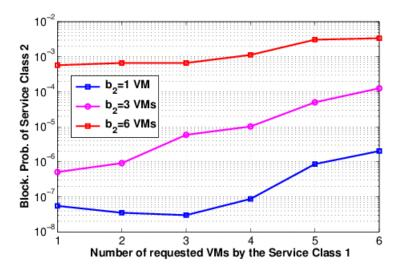
Figure 4.2: Blocking probability of the service class #2 versus the number of requested VM by the service class #1.
