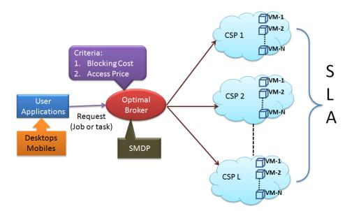
Figure 3.1: System model of Optimal Broker Design for Inter-Cloud Systems
