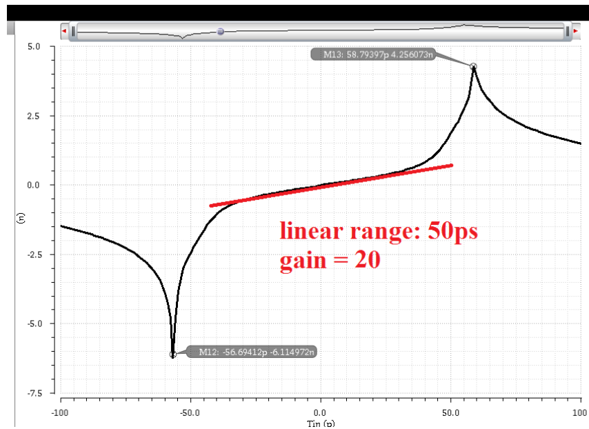
Figure 4.31: Time Amplifier Linear Range and Gain.
