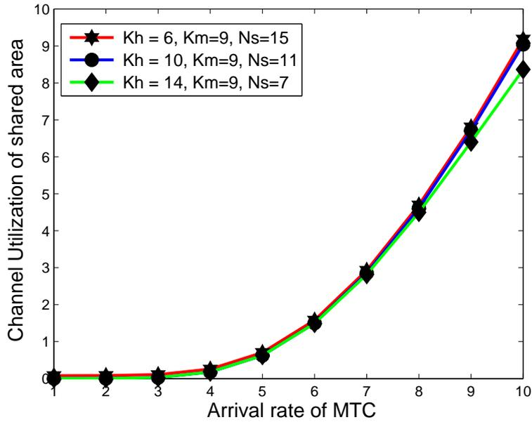
Figure 4.16: Channel Utilization of shared area vs. arrival rate of MTC with constant MTC threshold.
