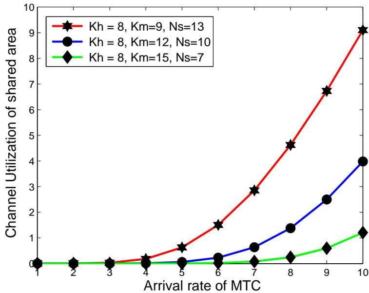
Figure 4.17: Channel Utilization of shared area vs. arrival rate of MTC with constant HTC threshold.
