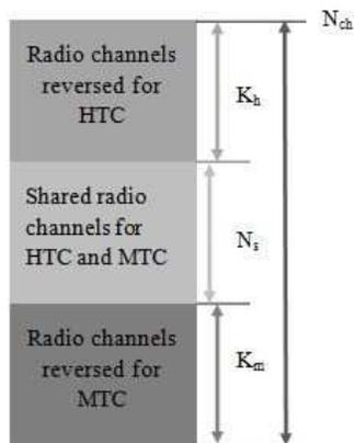
Figure 3.1: RRM scheme for HTC and MTC traffic.
