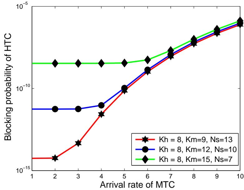
Figure 4.3: Blocking probability of HTC vs. arrival rate of MTC with constant HTC threshold.
