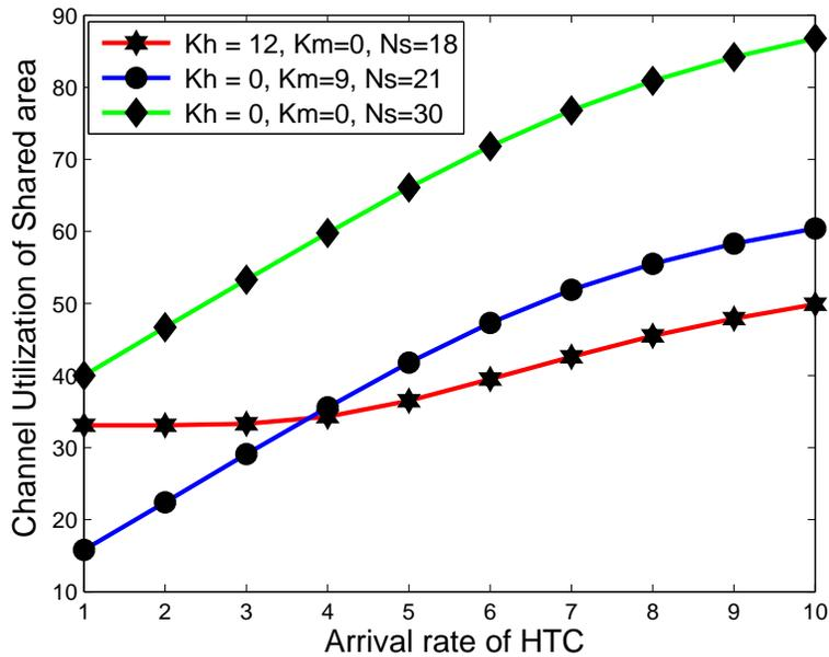
Figure 4.22: Channel Utilization of shared area vs. arrival rate of HTC without thresholds.
