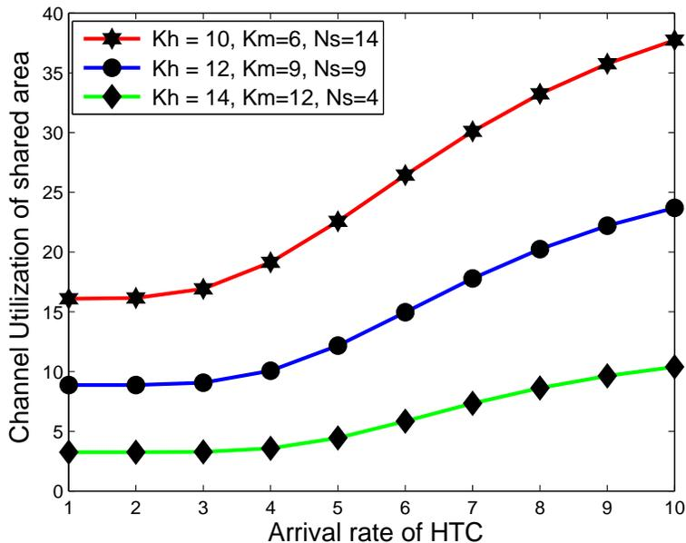
Figure 4.19: Channel Utilization of shared area vs. arrival rate of HTC with varied thresholds.
