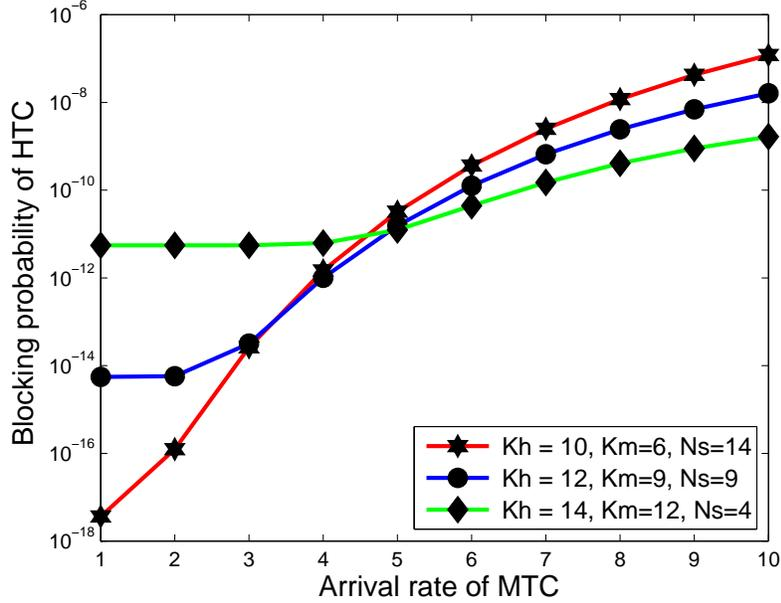
Figure 4.1: Blocking probability of HTC vs. arrival rate of MTC with varied thresholds.
