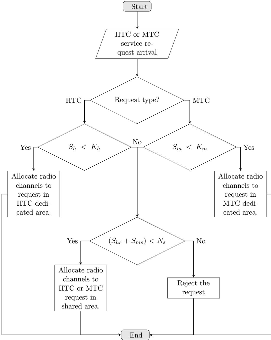
Figure 3.2: Flowchart of the proposed RRM scheme for HTC and MTC traffic.
