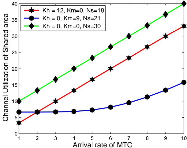
Figure 4.18: Channel Utilization of shared area vs. arrival rate of MTC without thresholds.
