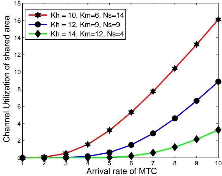
Figure 4.15: Channel Utilization of shared area vs. arrival rate of MTC with varied thresholds.
