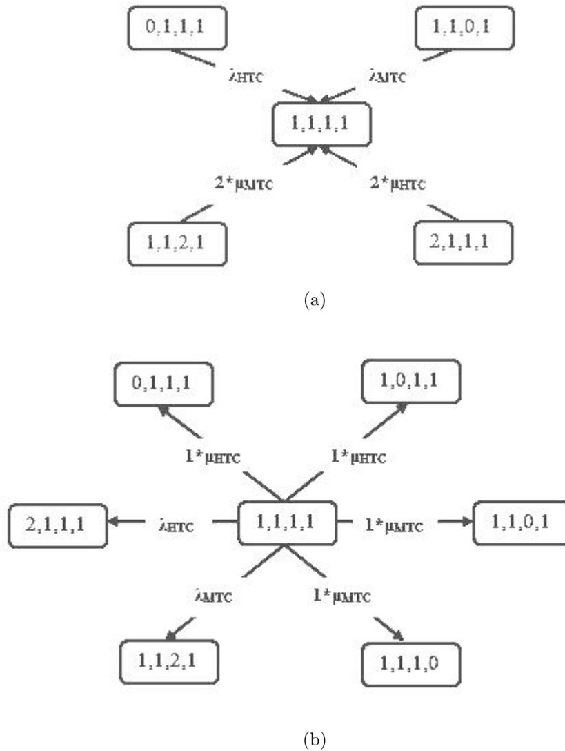
Figure 3.3: State transition diagram of state  $s$  of the CTMC model (a) Transitions to state  $s = (1, 1, 1, 1) \in S$  and (b) Transitions from state  $s = (1, 1, 1, 1) \in S$ .
