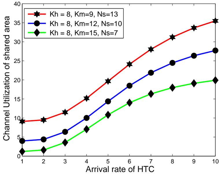
Figure 4.21: Channel Utilization of shared area vs. arrival rate of HTC with constant HTC threshold.
