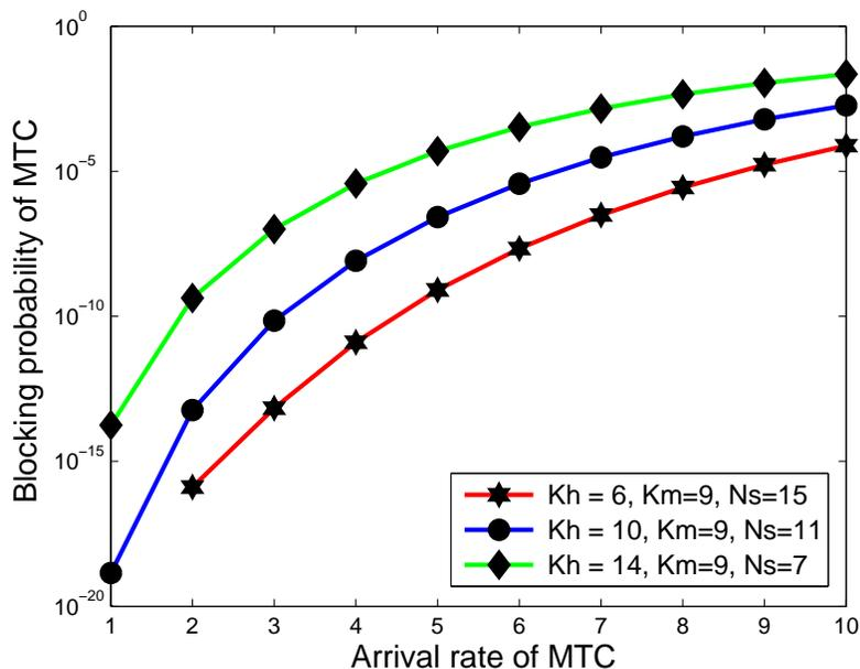
Figure 4.6: Blocking probability of MTC vs. arrival rate of MTC with constant MTC threshold.
