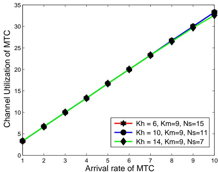
Figure 4.13: Channel Utilization for MTC vs. arrival rate of MTC with constant MTC threshold.
