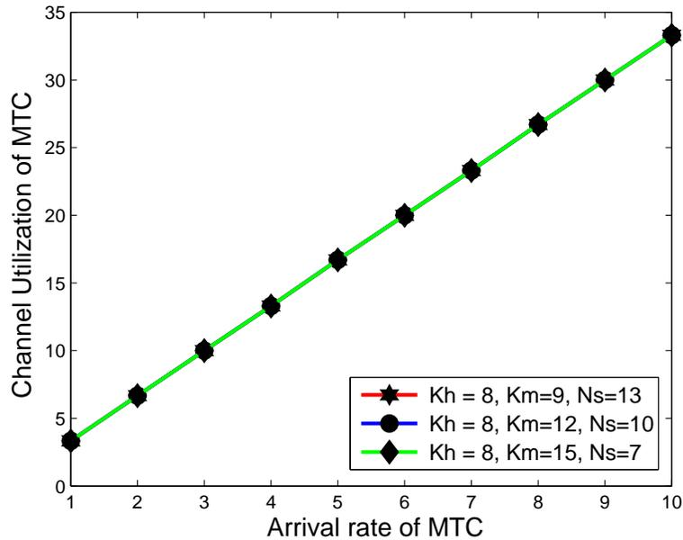
Figure 4.14: Channel Utilization for MTC vs. arrival rate of MTC with constant HTC threshold.
