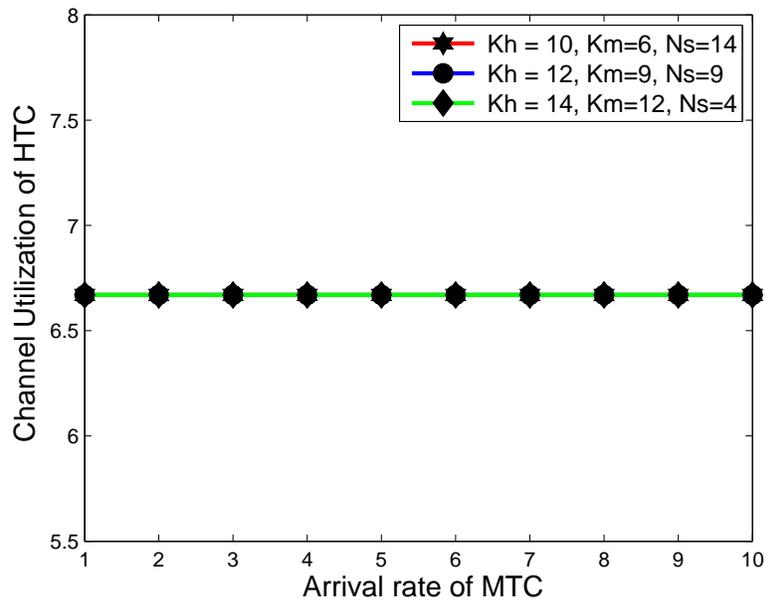
Figure 4.9: Channel Utilization for HTC vs. arrival rate of MTC with varied thresholds.
