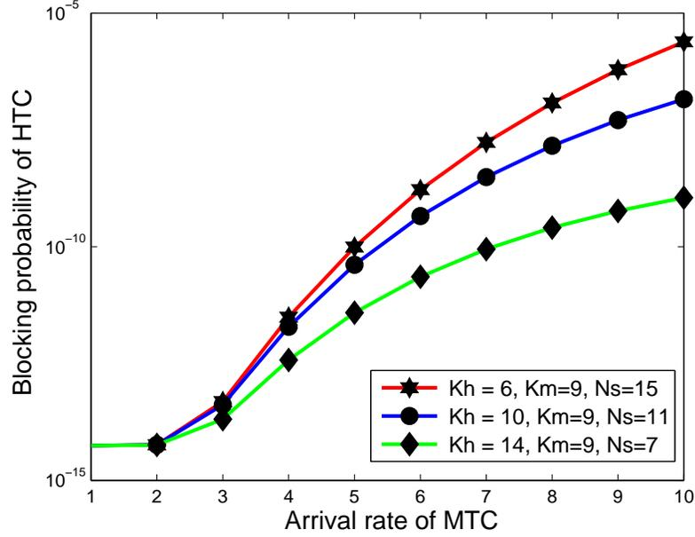
Figure 4.2: Blocking probability of HTC vs. arrival rate of MTC with constant MTC threshold.
