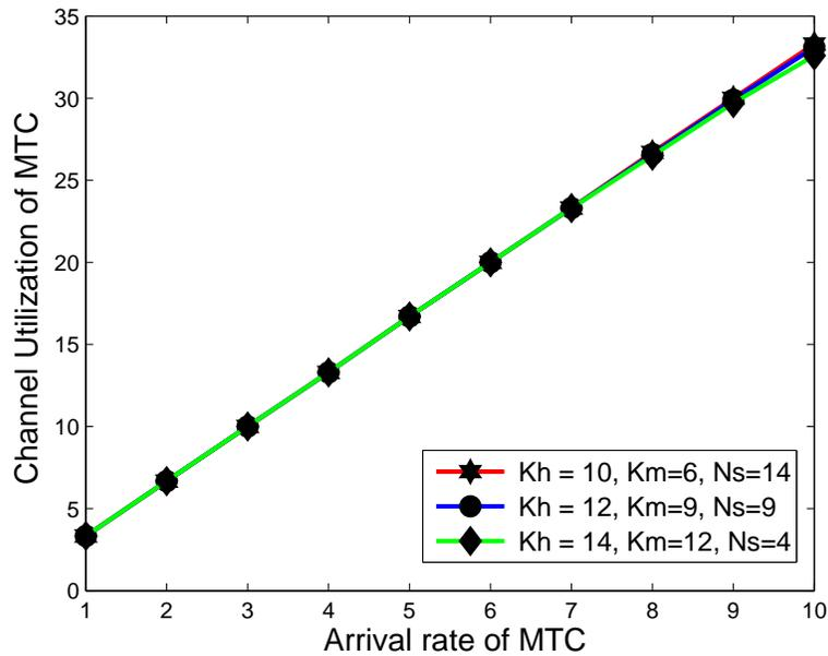
Figure 4.12: Channel Utilization for MTC vs. arrival rate of MTC with varied thresholds.
