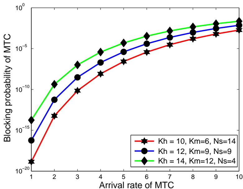
Figure 4.5: Blocking probability of MTC vs. arrival rate of MTC with varied thresholds.
