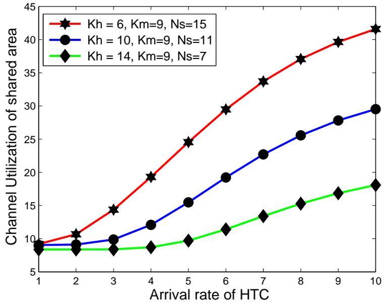
Figure 4.20: Channel Utilization of shared area vs. arrival rate of HTC with constant MTC threshold.
