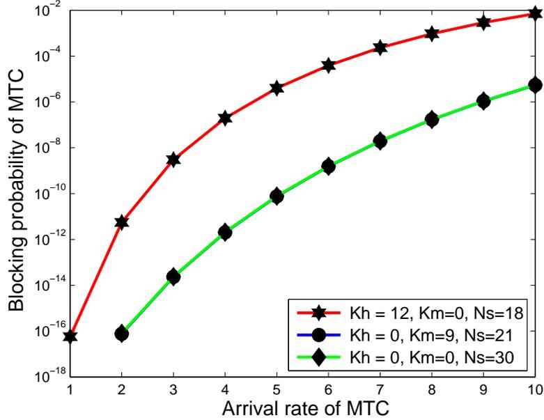
Figure 4.8: Blocking probability of MTC vs. arrival rate of MTC without thresholds.
