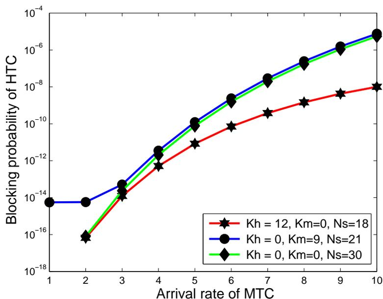
Figure 4.4: Blocking probability of HTC vs. arrival rate of MTC without thresholds.
