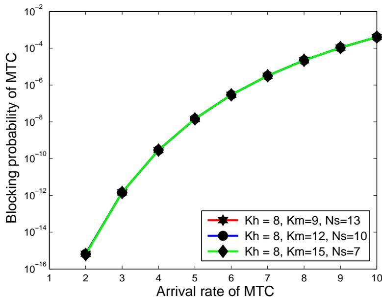
Figure 4.7: Blocking probability of MTC vs. arrival rate of MTC with constant HTC threshold.
