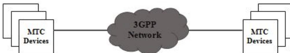
Figure 2.3: MTC Devices communicating directly with each other.
