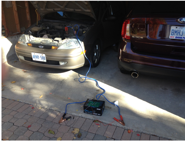
Figure 3.15: External PLC modem connection transmitter side
