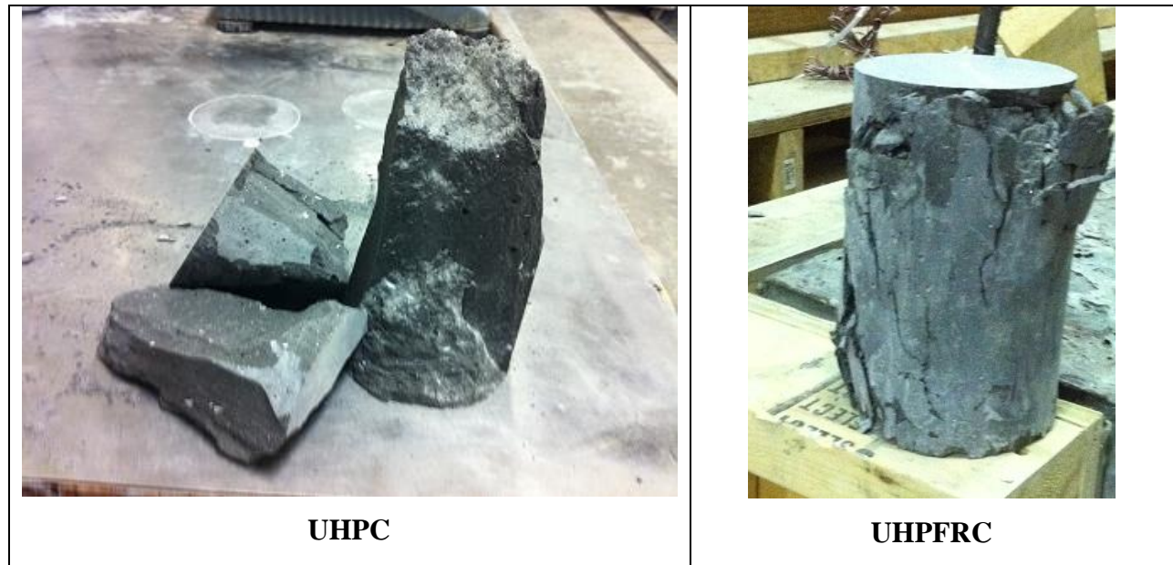
Figure 4.1 Failure modes of concrete cylindrical specimens under compression loading test
