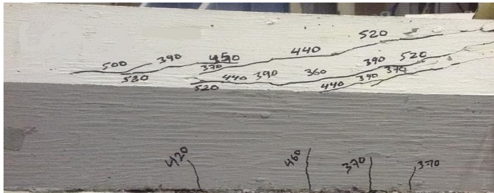
Figure 5.26 Crack pattern after failure – Beam UNS3-2
