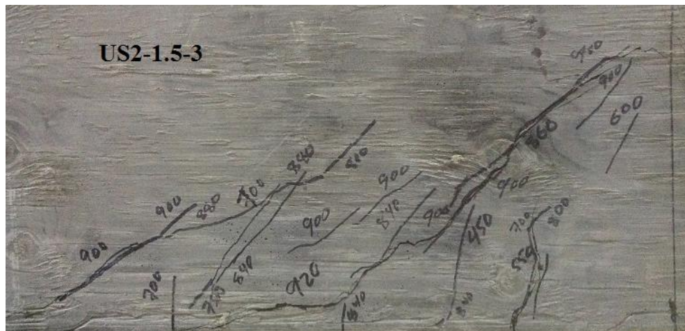
Figure 4.35 Crack pattern after failure – Beam US2-1.5-3.0
