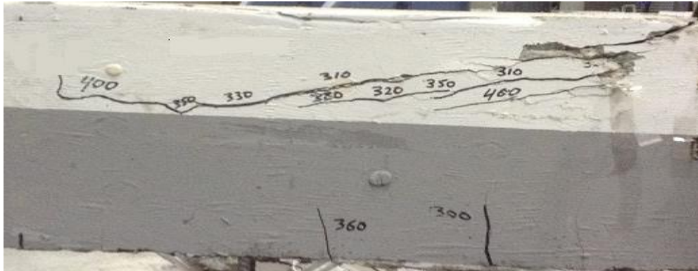
Figure 5.18 Crack pattern after failure – Beam UNS3-1.5
