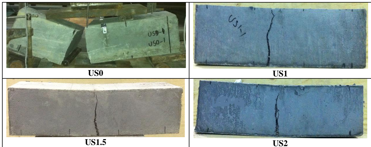
Figure 4.3 Flexural behaviour of UHPFRC prisms
