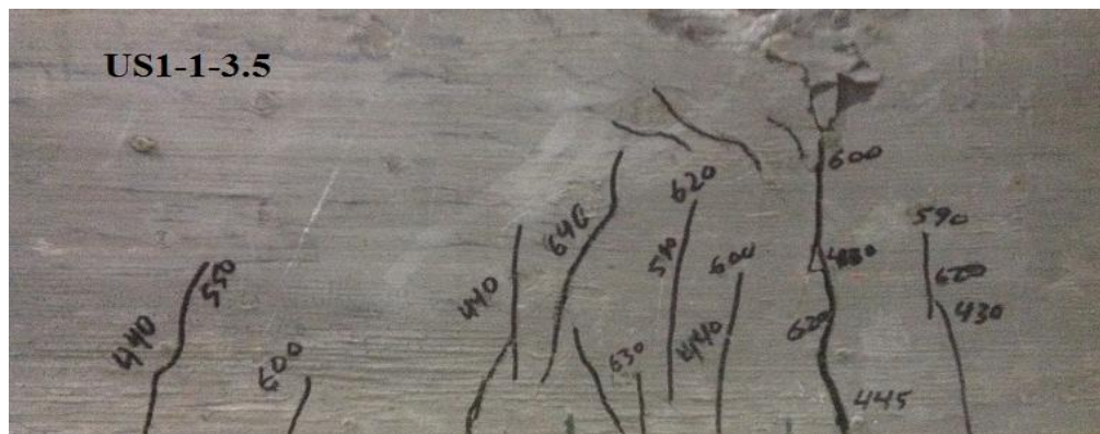
Figure 4.14 Crack pattern after failure – Beam US1-1-3.5
