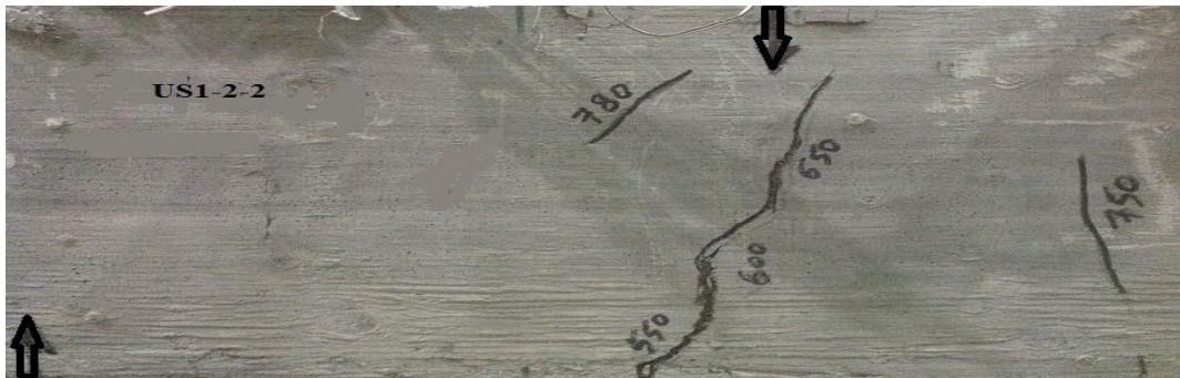
Figure 4.20 Crack pattern after failure – Beam US1-2-2.0
