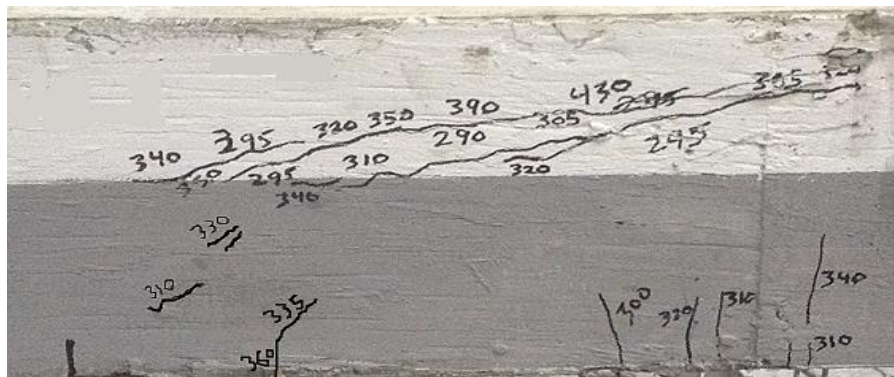
Figure 5.6 Crack pattern after failure – Beam UNS3-1
