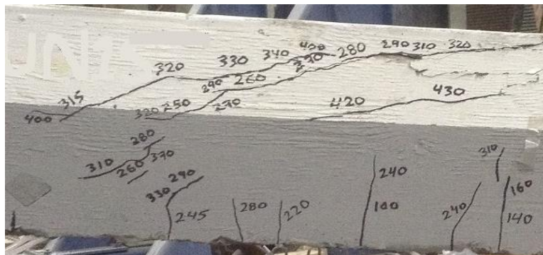
Figure 5.10 Crack pattern after failure – Beam UNS3-1S
