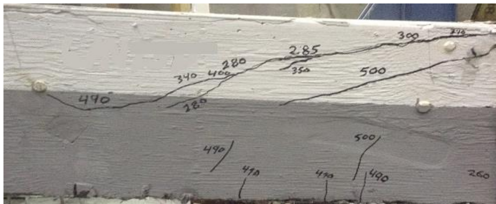
Figure 5.20 Crack pattern after failure – Beam UNS3-1.5D
