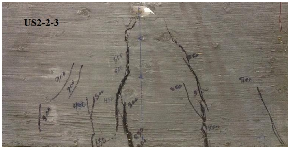
Figure 4.38 Crack pattern after failure – Beam US2-2-3.0
