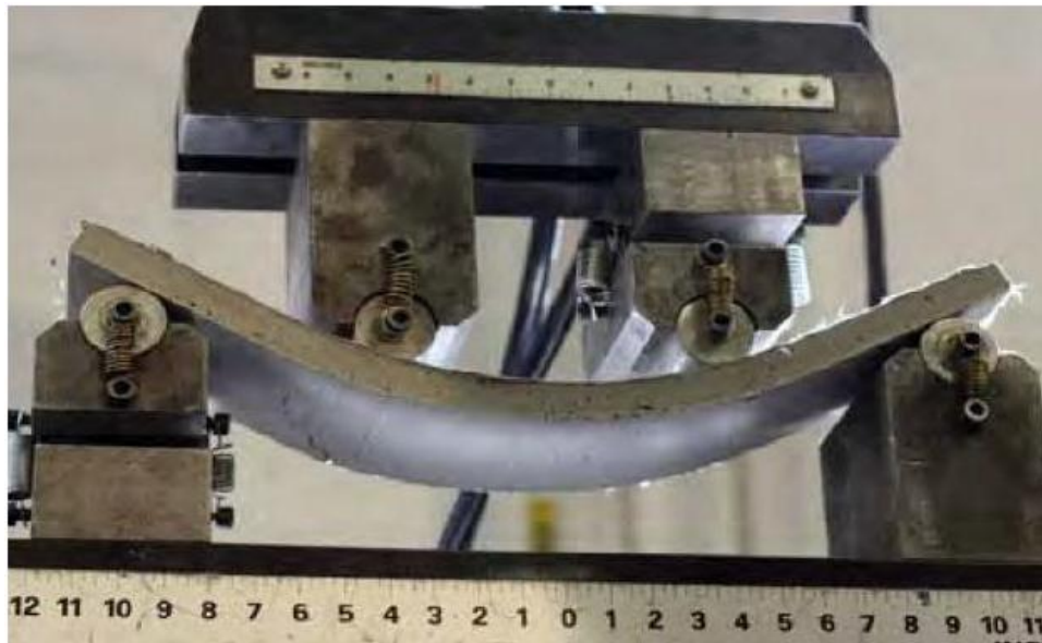
Figure 2.4: Ductile Response of ECC under Flexural Loading (Li 2011)
