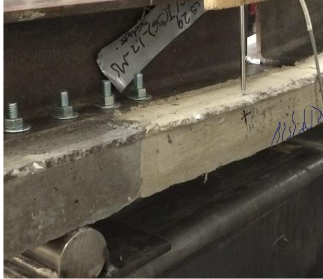
Figure 4. 12: Crack Characterization in Transition Zone
