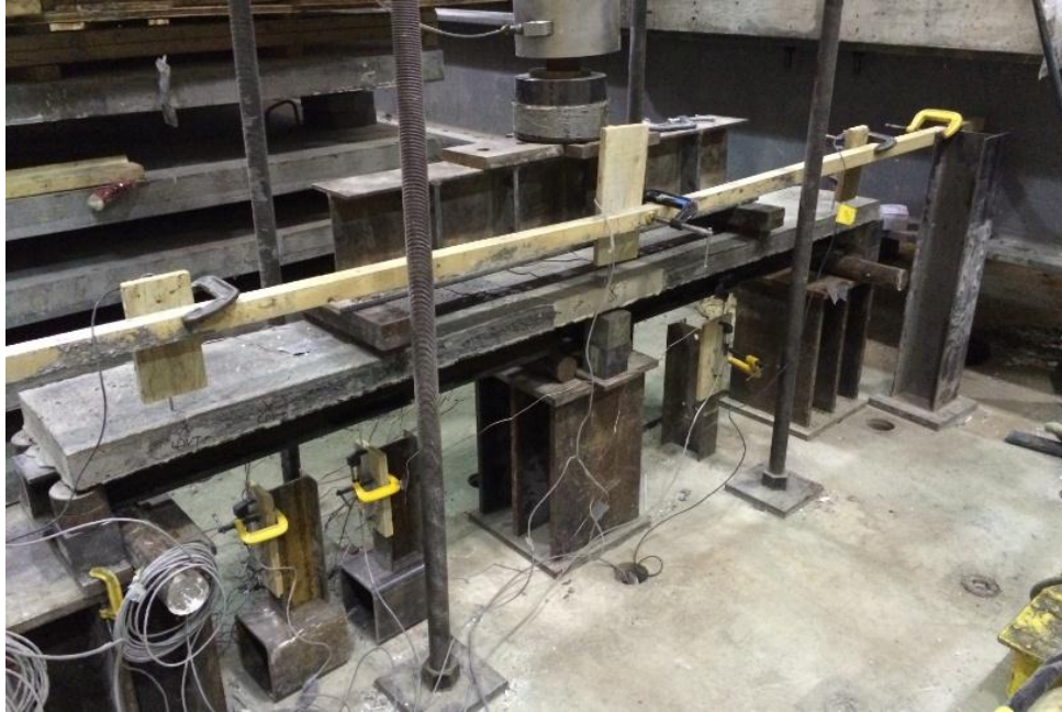
Figure 3.13: Testing Instrumentation of 1/6 th Scale Full Bridge Model
