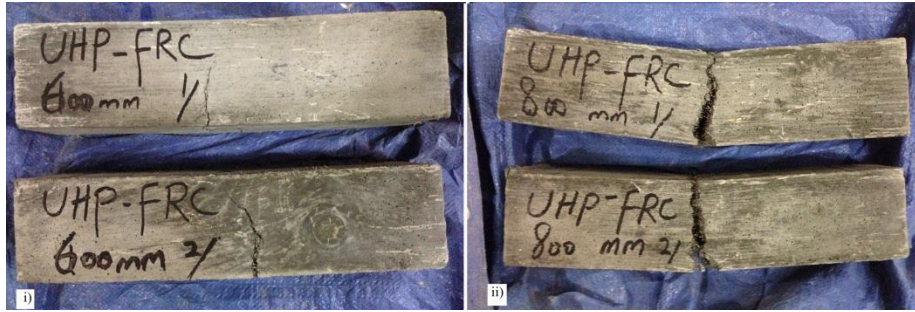
Figure 4.10: UHP-FRC Prisms After Impact Test; i) 600 mm and ii) 800 mm
