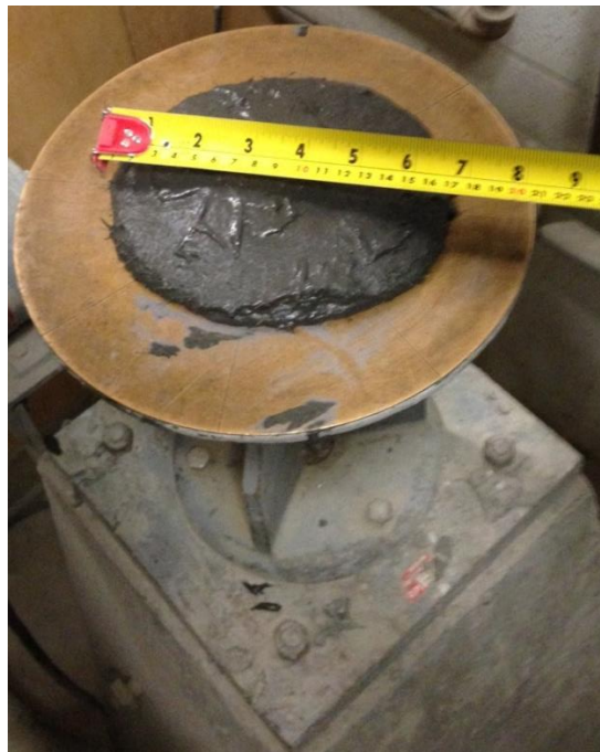
Figure 3.1: Slump Flow Test for EHP-FRC
