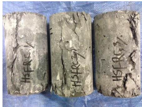
Figure 4.3: EHS-FRC Cylinders After Compressive Test
