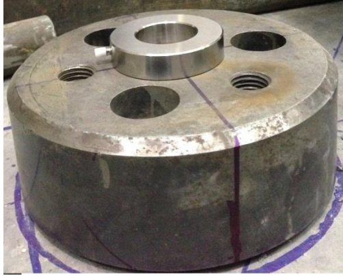
Figure 3.16: Location of the Dynamic Load Cell on Steel Cover
