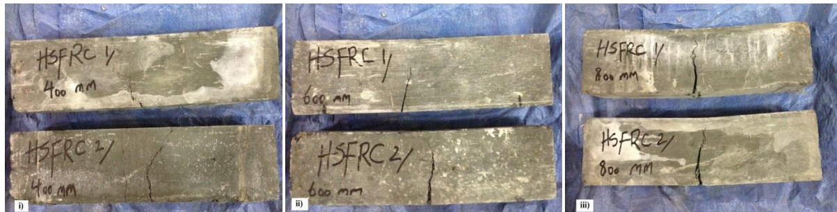
Figure 4.12: EHS-FRC Prisms after Impact Test; i) 400 mm, ii) 600 mm and iii) 800 mm
