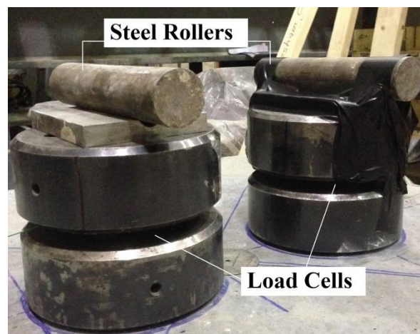
Figure 3.17: Position of the Dynamic Load Cells, Steel Rollers and Steel Covers
