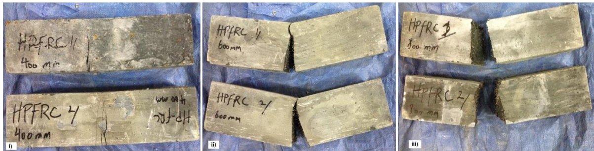
Figure 4.11: EHP-FRC Prisms After Impact Test; i) 400 mm, ii) 600 mm and iii) 800 mm
