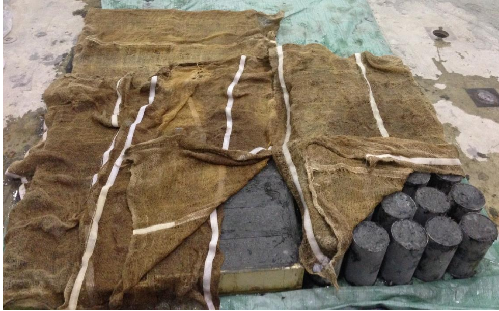
Figure 3.3: Covered Samples with Damp Burlap During First Three Days
