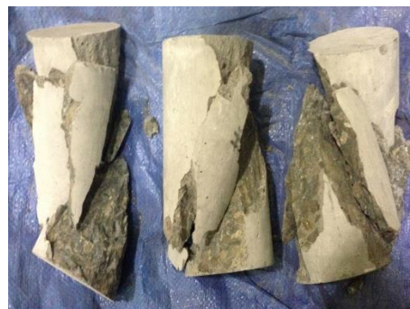
Figure 4.4: HSC Cylinders After Compressive Test
