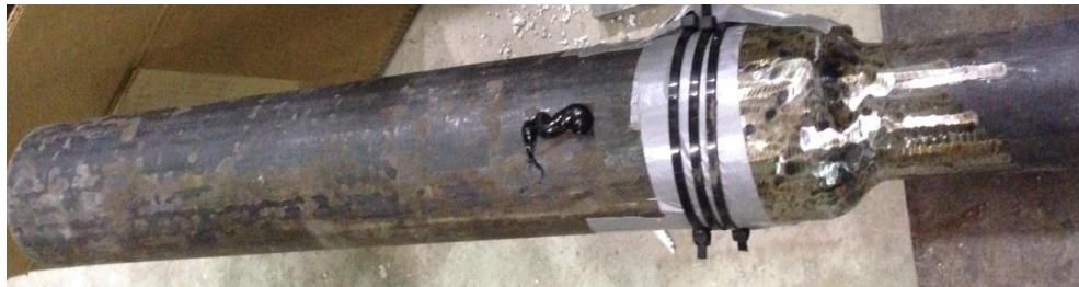
Figure 3.20: Applied Rubber on Drop Weight Before Mounting Accelerometer
