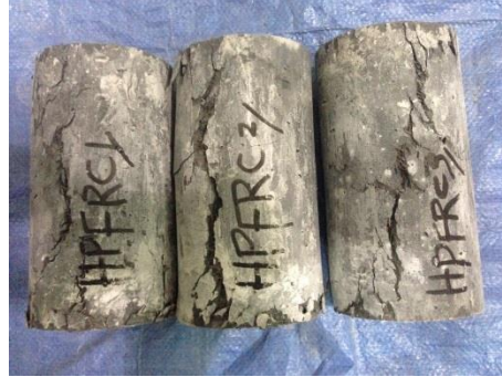
Figure 4.2: EHP-FRC Cylinders After Compressive Test
