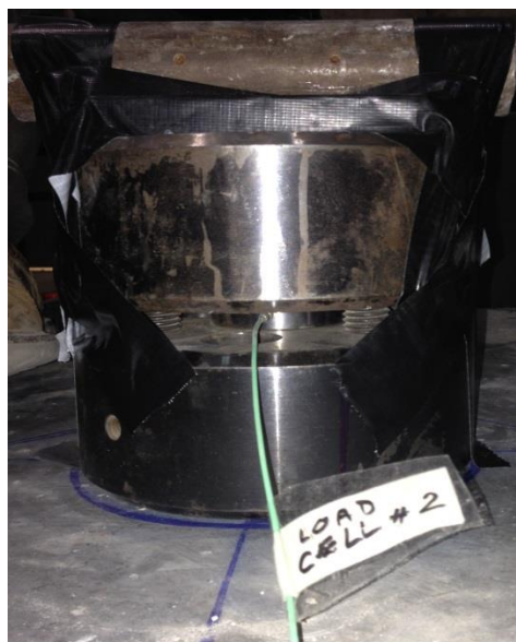
Figure 3.18: Settled Dynamic Load Cell Between Steel Covers
