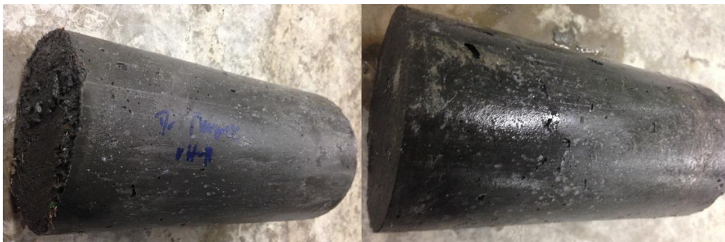
Figure 3.6: Cylinder Specimens Before and After Grinding
