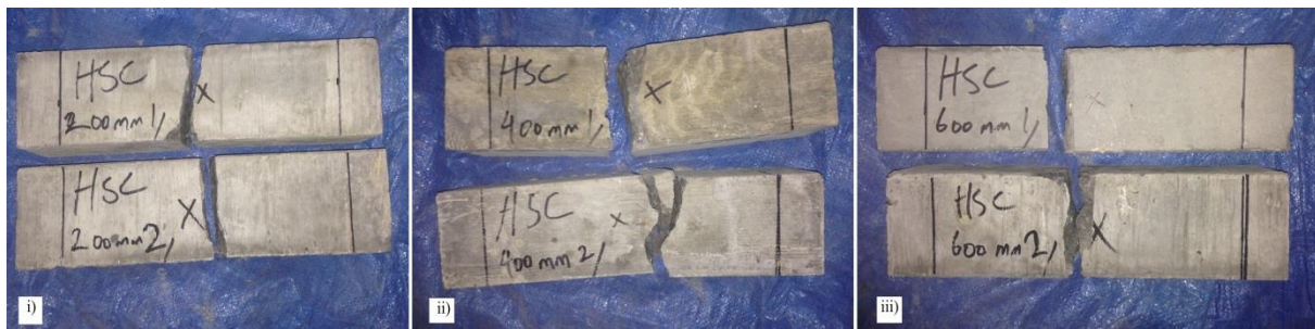
Figure 4.13: HSC Prisms After Impact Test; i) 200 mm, ii) 400 mm and iii) 600 mm
