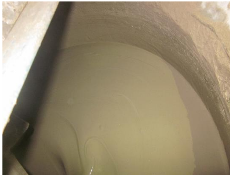
Fig. 3.4:- ECC production in the mixer machine
