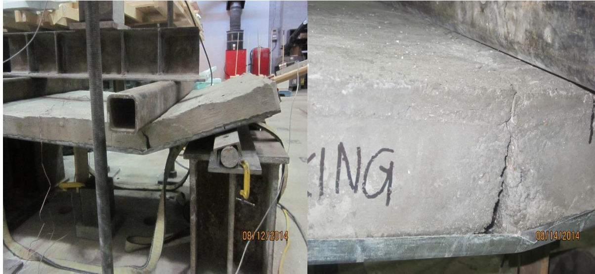
Fig. 3.8:- Cracking and steel-concrete separation of composite slab
