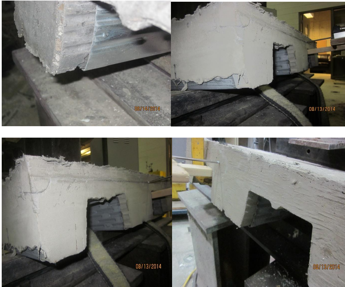
Fig. 3.10:- End slip between steel sheet and concrete in composite slabs
