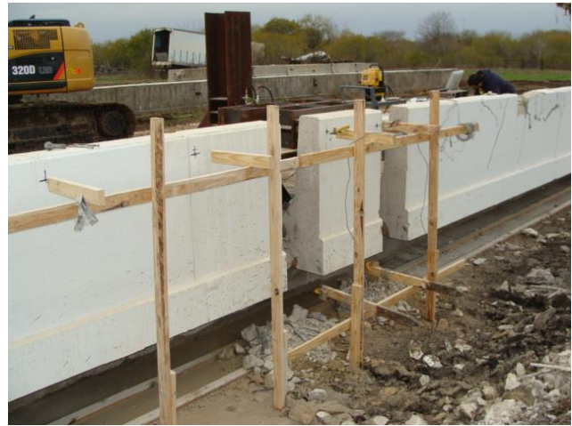
(c) Cantilever test over 1-m over length
