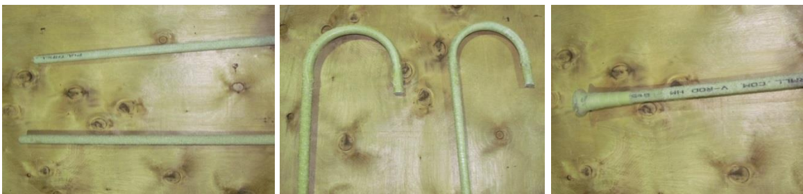
Figure 3. 1 Views of sand-coated GFRP bars; straight (left), 180°-hook (middle) and headed (right) bars
