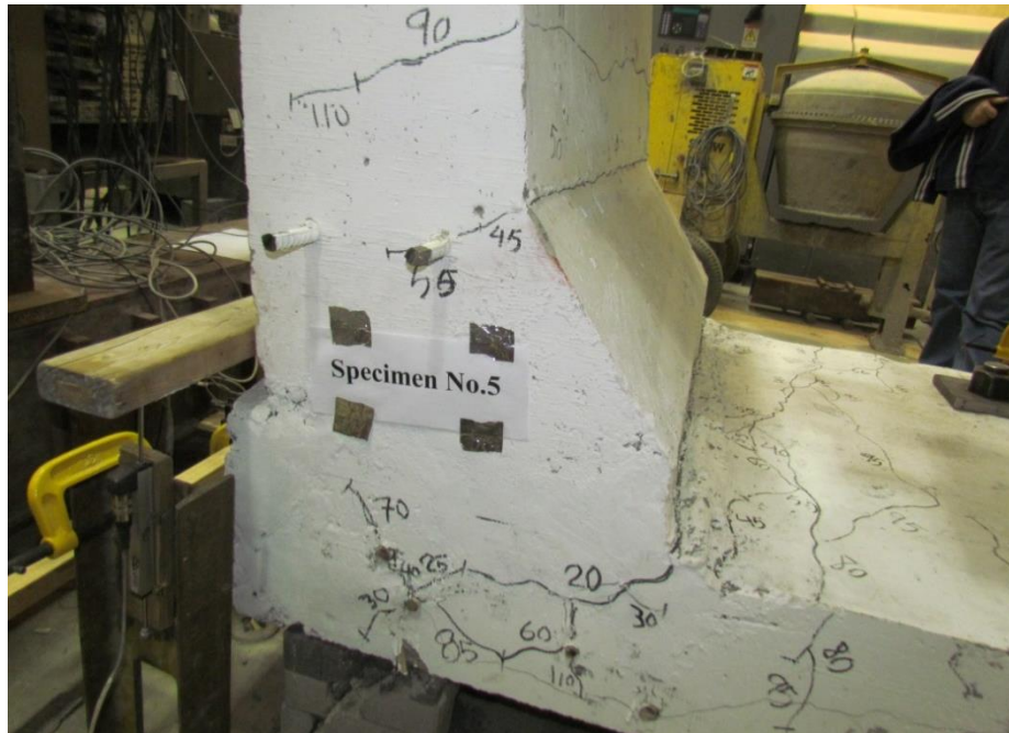
d) Close-up view of crack pattern at the barrier-deck junction from the left Figure 4. 20 View of the crack pattern in barrier Model 5 with steel reinforcing bars
