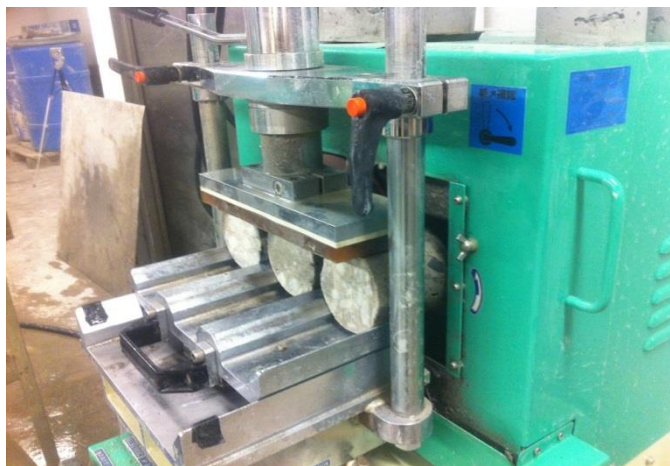
Figure B.5 Concrete cap grinding machine
