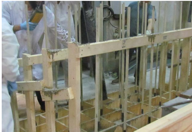
Figure 3. 26 View of concrete casting of the pullout cubes using plastic pipe
