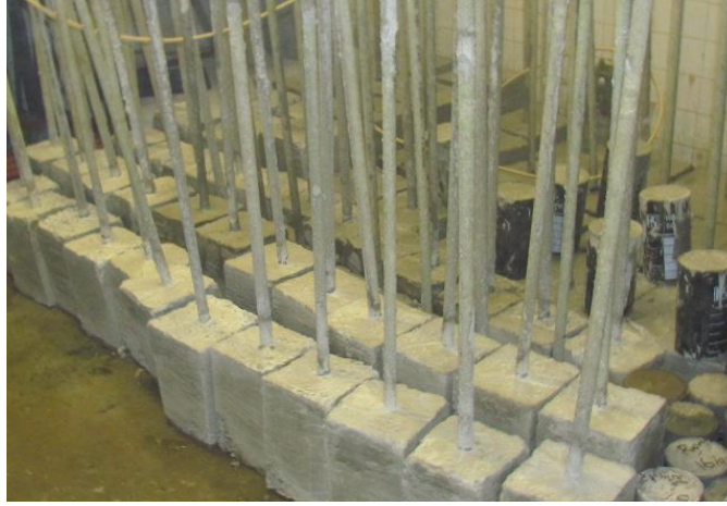
Figure 3. 28 View of concrete blocks after removal of formworks
