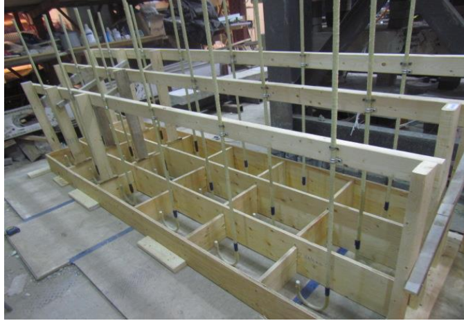
Figure 3. 25 Placement of GFRP hook bars in 300-mm x 500-mm concrete cubes
