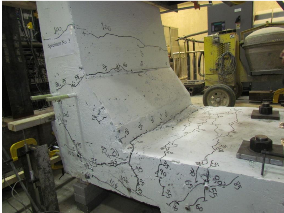
c) View of cracks at the deck and barrier wall from the left side
