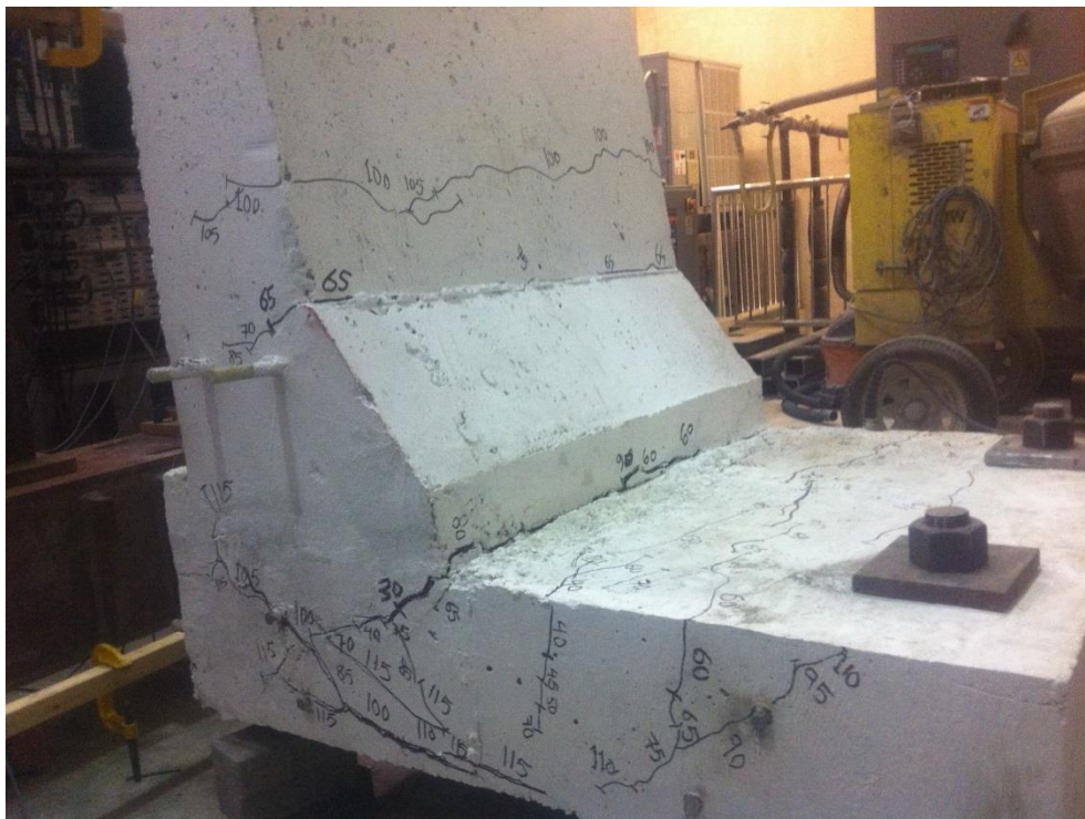
c) View of cracks in the deck and barrier wall from the left side
