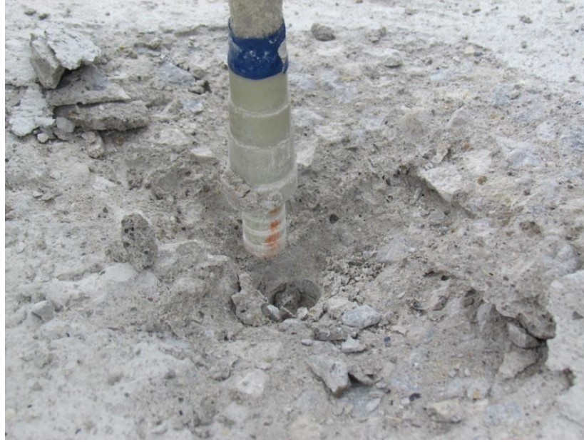
Figure 3. 57 Failure of GFRP headed-end showing broken head with end portion left in concrete
