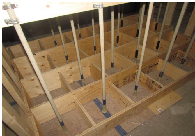
Figure 3. 24 View of GFRP headed-end bars embedded in 300-mm width cubes
