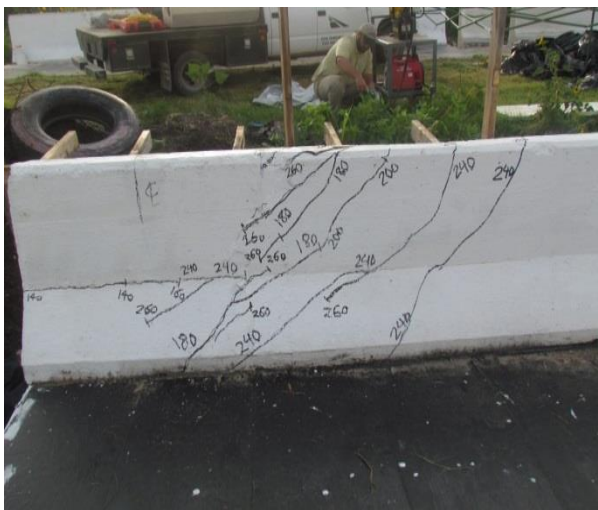
(a) Crack pattern at front face
