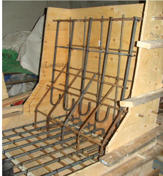
Figure 4. 9 View of steel bars arrangement in barrier Model 5
