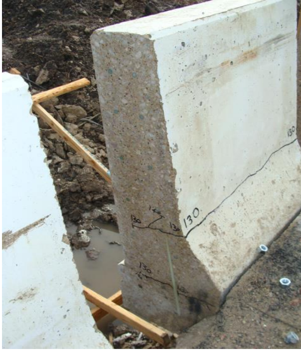
(a) Cracks at front face
