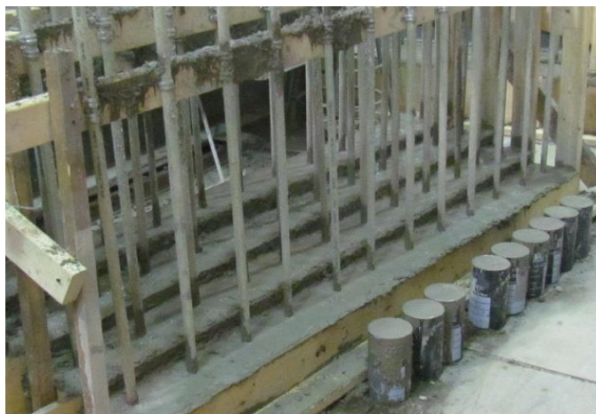
Figure 3. 27 Photo of cast concrete in 150-mm width cubes with cylinders cured next to the specimens
