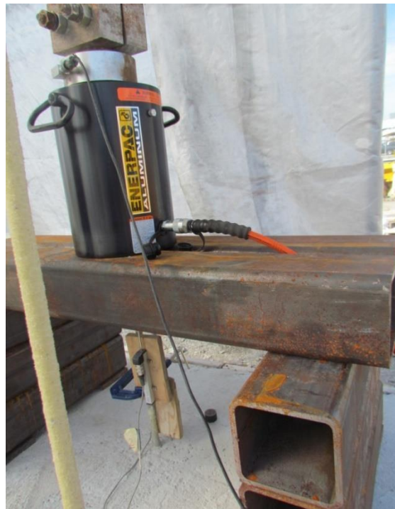
Figure 3. 32 View of single GFRP bar test setup for concrete slab specimens
