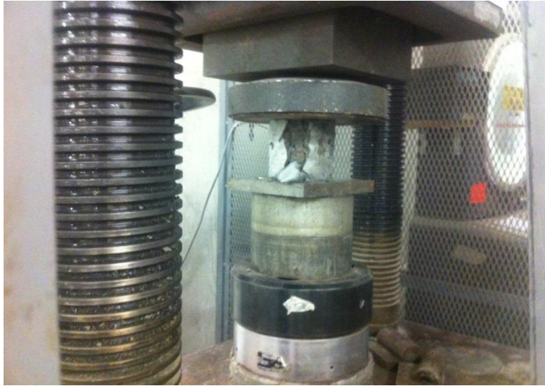
Figure B.6 Concrete compressive strength testing machine during testing
