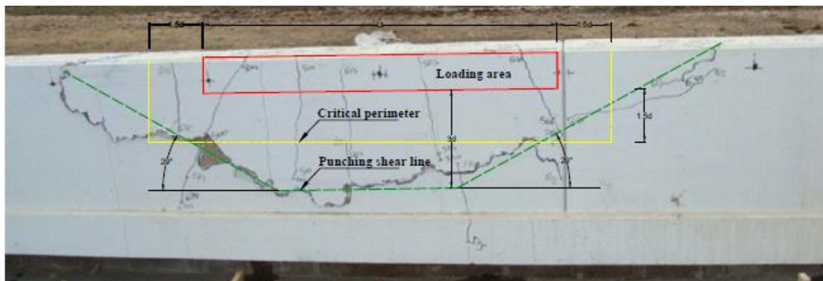
(b) Punching shear region at back face of the wall
