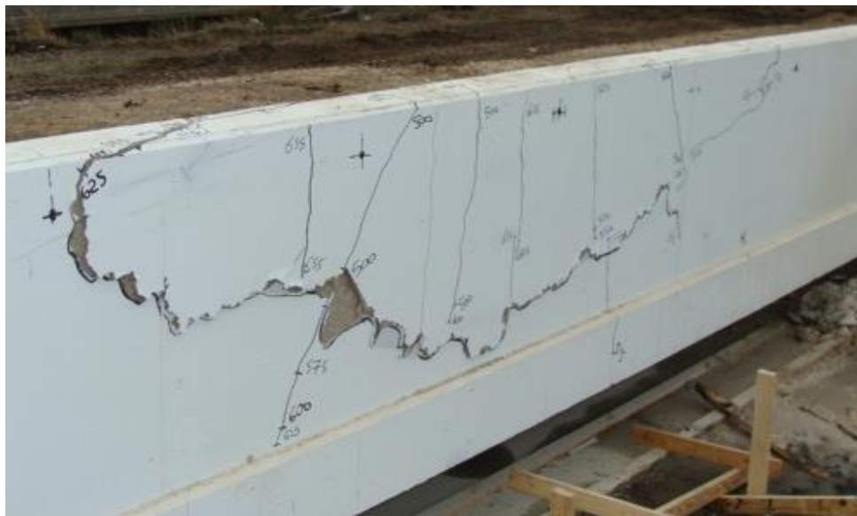
e) Crack pattern at the barrier back face
