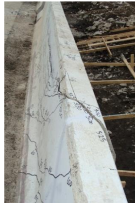
c) Side view of punching shear
