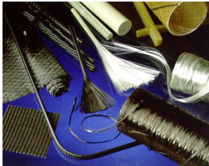
Figure 2. 1 Various types of FRPs for reinforcement and rehabilitating concrete structures (Adopted: ISIS Canada Module 3, 2006)
