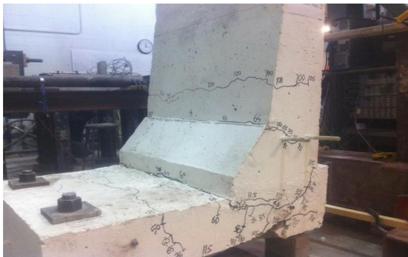
a) View of cracks in the barrier and deck from right side
