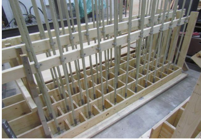
Figure 3. 22 Placement of GFRP straight and headed-end bars in 150-mm width cubes
