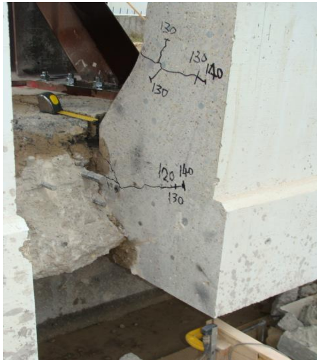
(b) Close up view of corner cracks
