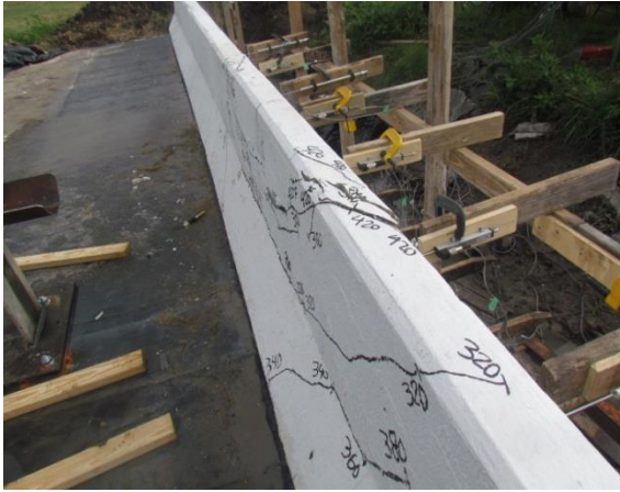
(c) Punching shear failure on top of the wall
