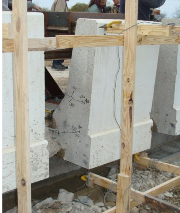
(b) Extended corner cracks
