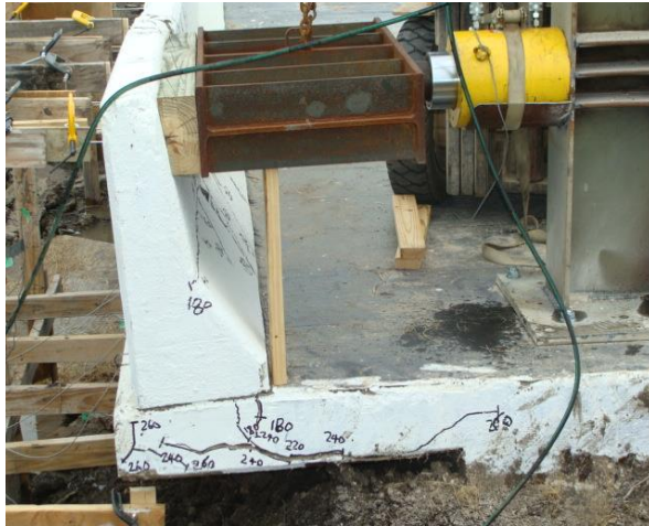
(c) Corner diagonal tension crack
