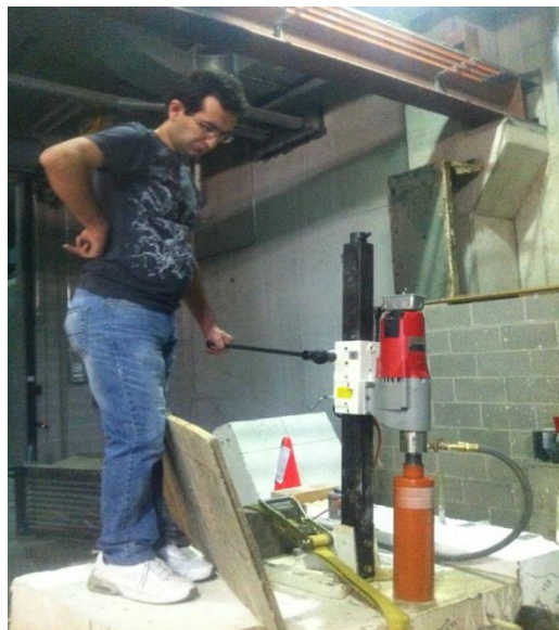
Figure B.2 Core sampling of the tested barrier wall
