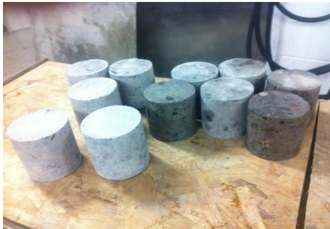
Figure B.4 Image of core samples after cutting and grinding
