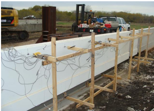
Figure 5. 21 Views of test setup for static testing of the barrier wall at interior and exterior locations over 2.4-m length and cantilever test over 1-m length
