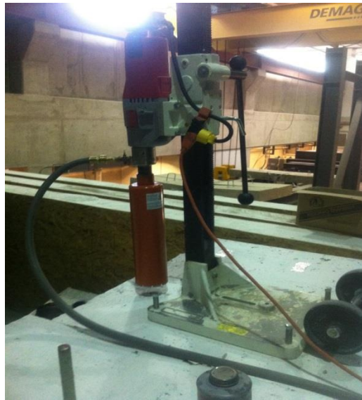
Figure B.1 Photo of core sampling machine
