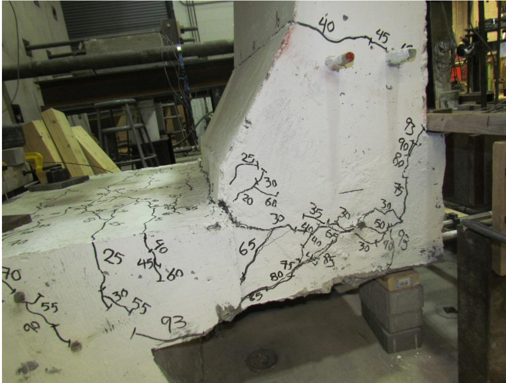
b) Close-up view of crack pattern at barrier-deck junction (right view)
