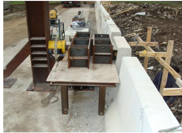
Figure 5. 21 Views of test setup for static testing of the barrier wall at interior and exterior locations over 2.4-m length and cantilever test over 1-m length
