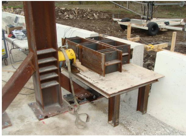
Figure 5. 21 Views of test setup for static testing of the barrier wall at interior and exterior locations over 2.4-m length and cantilever test over 1-m length
