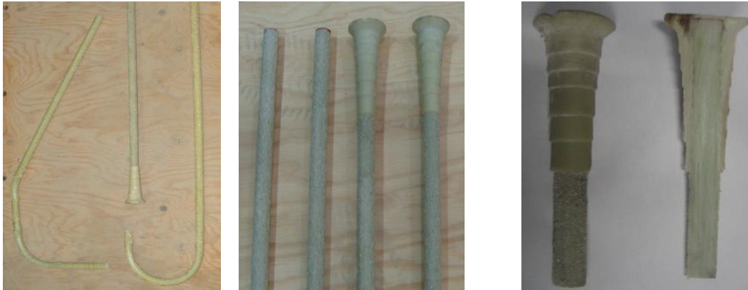
Figure 3. 2 Views of GFRP sand-coated HM and SM bars Figure 3. 3 View of headed-end bar
