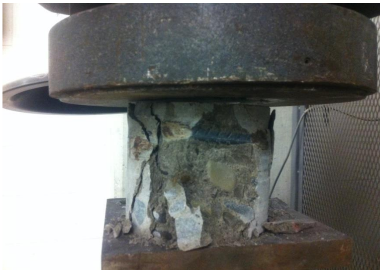
Figure B.7 Close-up view of tested concrete core showing presence of steel bar in the core sample
