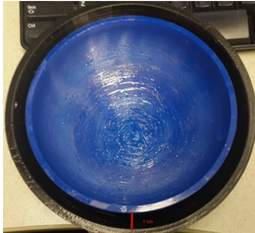
Figure 5-1 Two hemispheres inside each other to mold the layers of phantoms. The read line is the gap between the two bowls that is 1cm.
