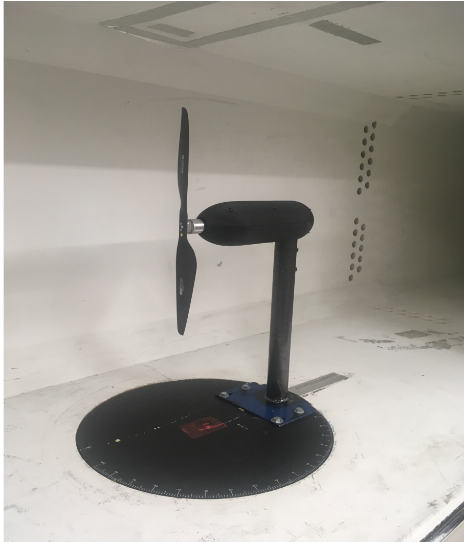
Figure 3.3: Test stand mounted on wind tunnel turntable with cowling on.
