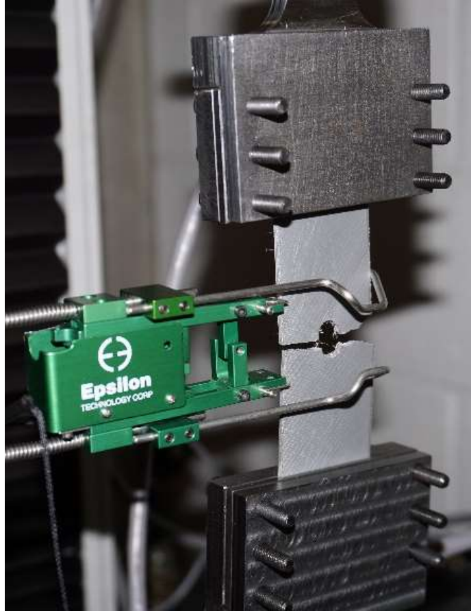
Figure 3.11. A variable stiffness specimen ( w/D=4 ) after failure (LGM mode).
