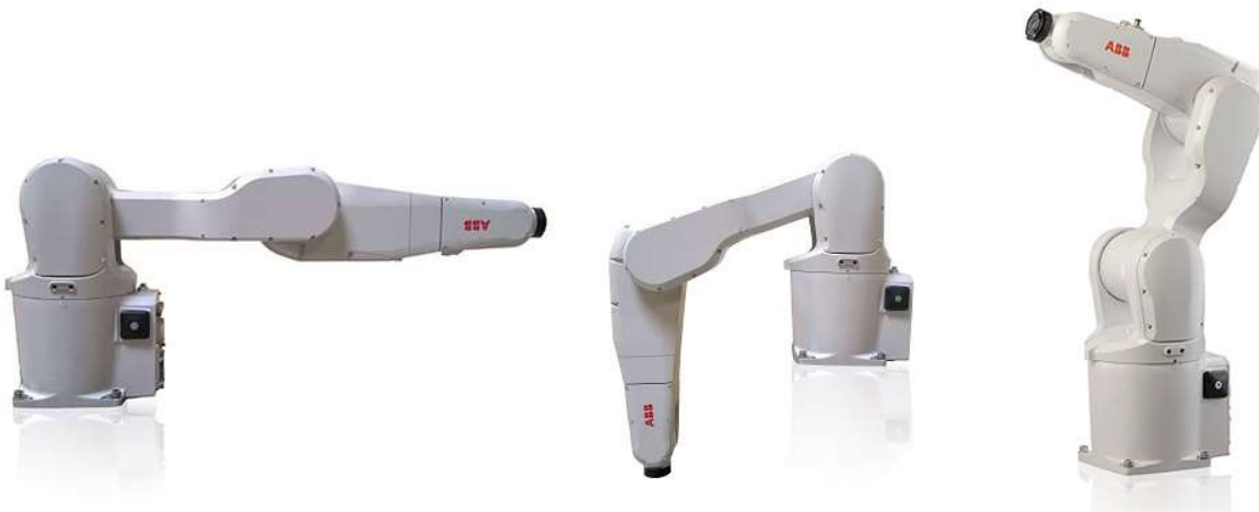
Figure 5.1 ABB IRB1200 Industrial Robot demonstrating degrees of freedom
