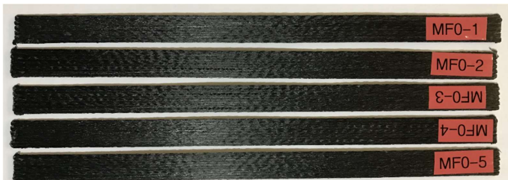
Figure 6.8 ASTM D3039 Tensile test coupons manufactured with Markforged Continuous Carbon Fiber
