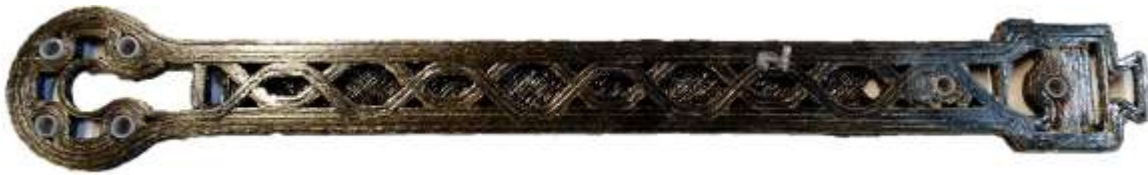
Figure 2.8 Drone arm printed using continuous carbon fiber [31]
