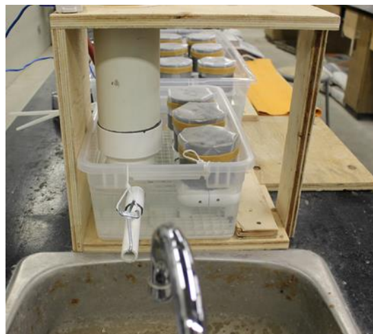
Fig. 2. Testing apparatus used in the determination of sorptivity
