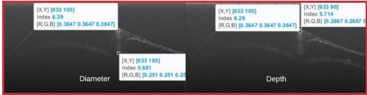
Figure 5.3 Depiction of point-picking for measuring vessel diameter and vessel depth. In this case the diameter and depth of the vessel was 80 and 15 pixels respectively. Dots represent pixels for which data is being displayed.
