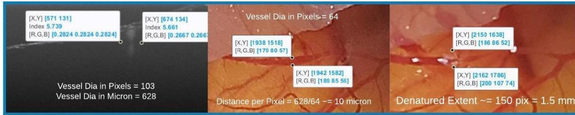
Figure 5.5 Depiction of HAZ point picking. From left to right: a structural OCT image followed by two photographs. The lateral natural extent of the vessel is firstly acquired in structural image pixels. By multiplying by the lateral distance per pixel ( 6.1 \mu\text{m} ) the natural extent of the vessel is then acquired in micrometers. The natural extent of the vessel is then measured in photograph pixels and thus the distance per photograph pixel is known. The denatured extent is then measured in photograph pixels, by multiplying this value by the distance per photograph pixel the denatured extent can be acquired in micron. The HAZ is then calculated by subtracting the natural extent of the vessel from the denatured extent. In this case \text{HAZ} = 872 \mu\text{m} . Dots represent pixels for which data is being displayed.
