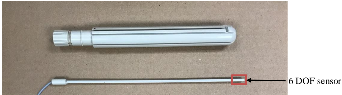
Figure 8. Disassembled 6 DOF tracked vaginal cylinder.
