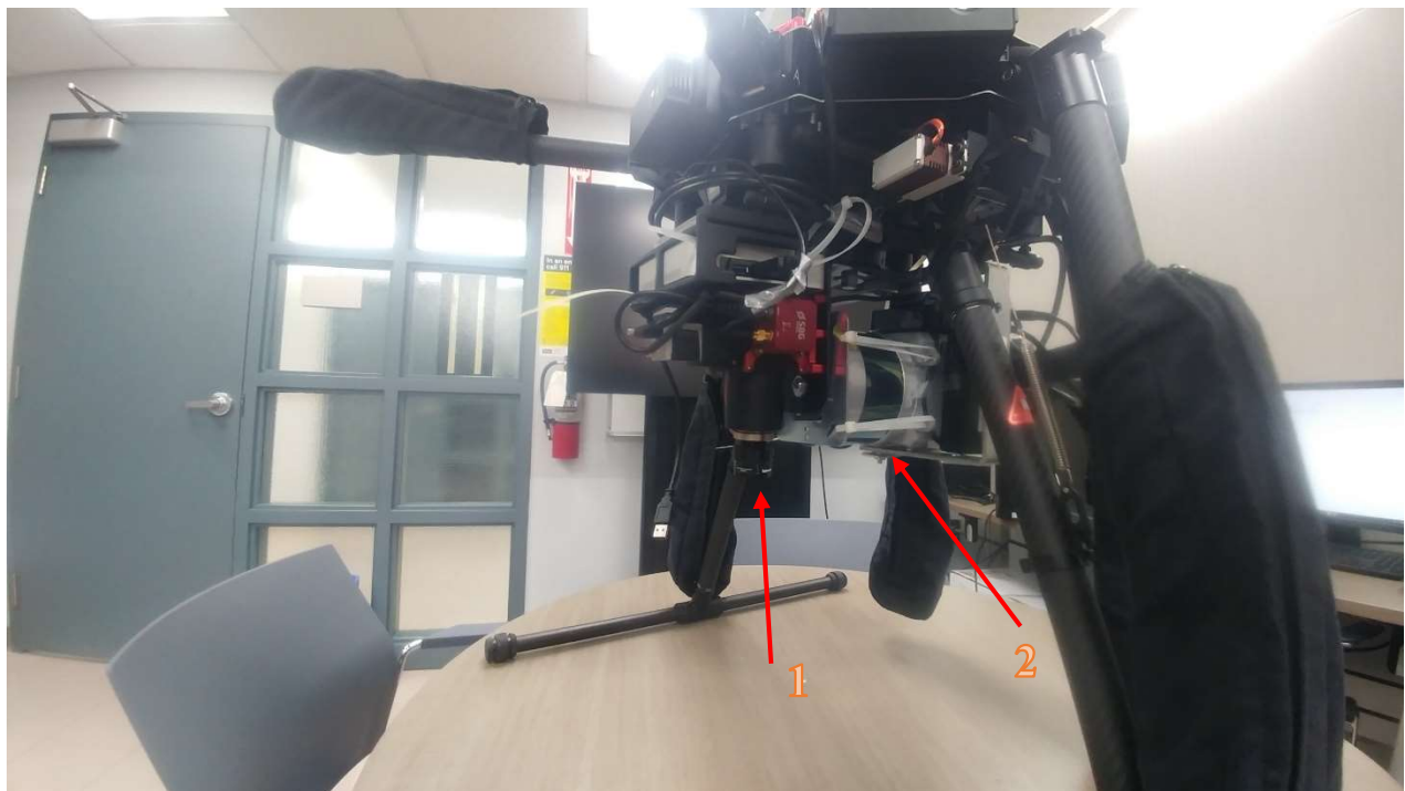
Fig 6.2: The System mounted in ULS mode with Hyperspectral camera
