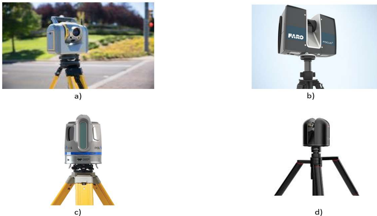
Fig 2.10: Examples of different STLS, a) Trimble SX10, b) Faro Focus-350 c) Optech Polaris, and d) Leica BLK360
