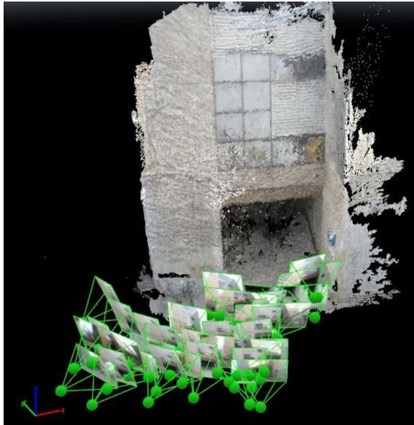
Fig 5.11: EPH façade SfM point cloud (images positions are the green circles)
