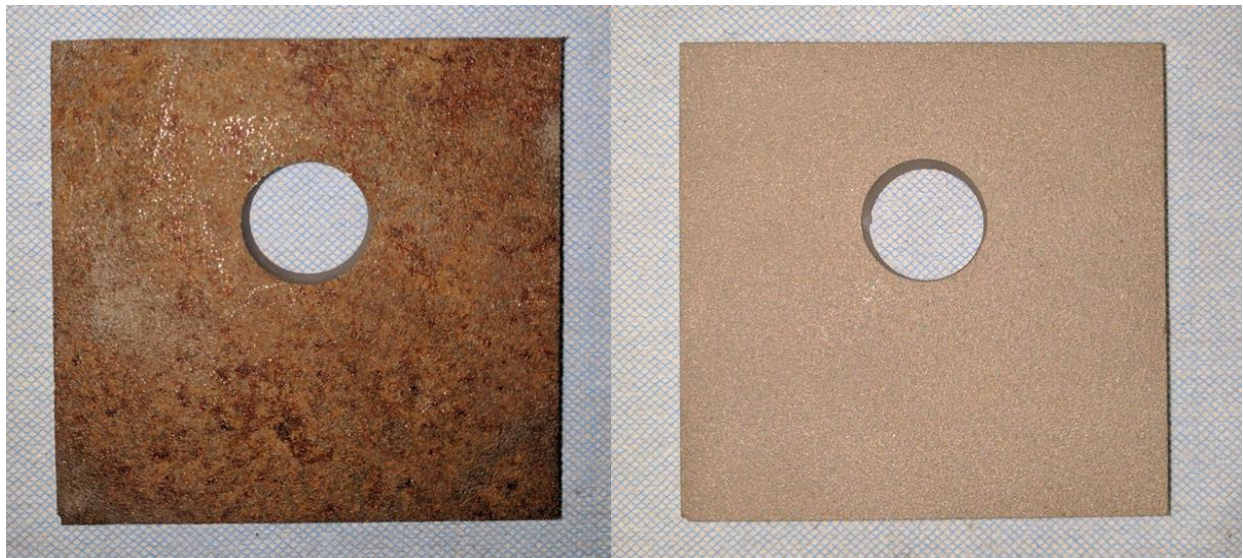
Figure 3-3: Specimen Before and After Blast Cleaning with Stainless Steel Grit
