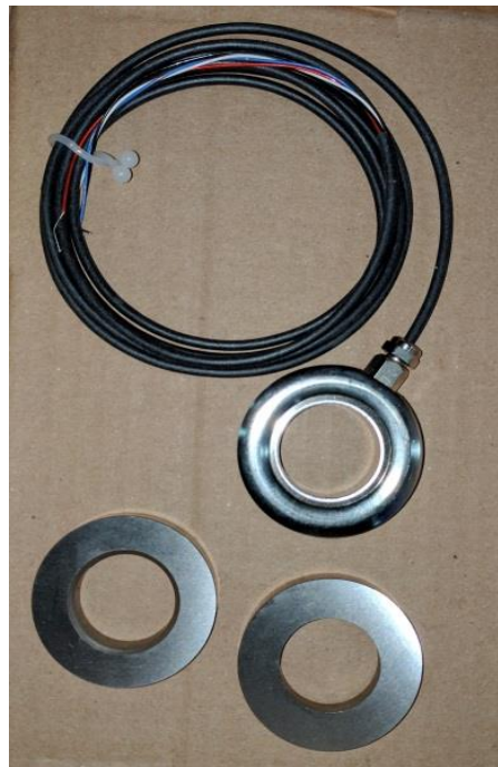
Figure 3-10: Photo of Washer Type Load Cell for Measuring Clamping Force
