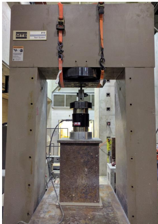
Figure 3-17: View of the MTS Machine with Slip Resistance Test Set-Up
