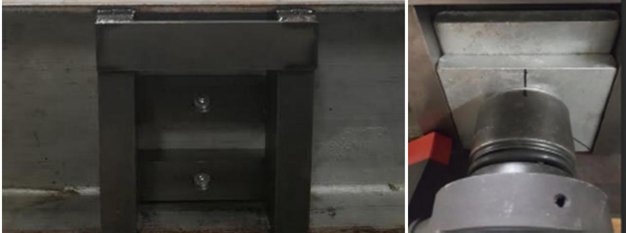
Figure 3-13: Specially manufactured jig and plate assembly for the turn-of-nut clamping method (Cameron, 2017)
