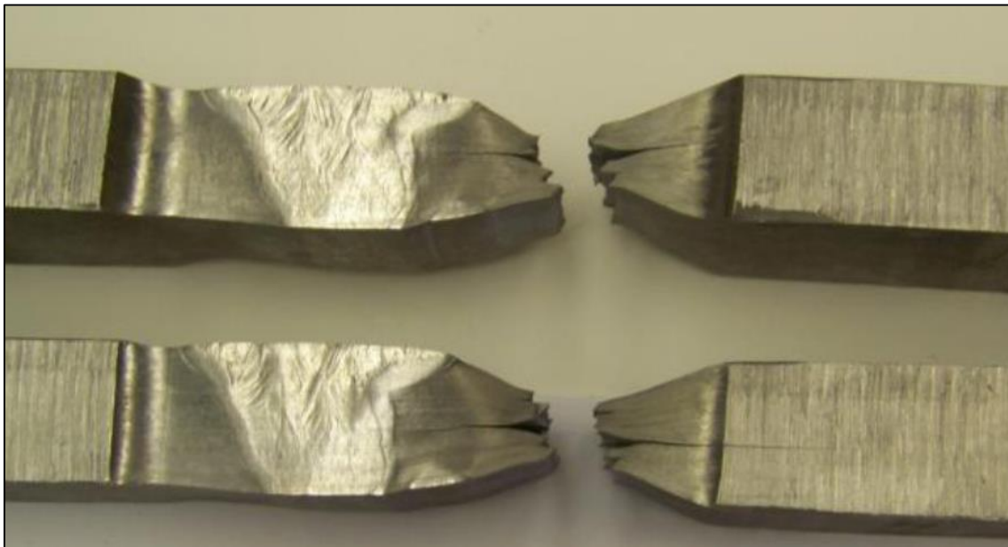
Figure 2-39: Welded A1010 Transverse Tensile Samples (Seradj, 2010)
