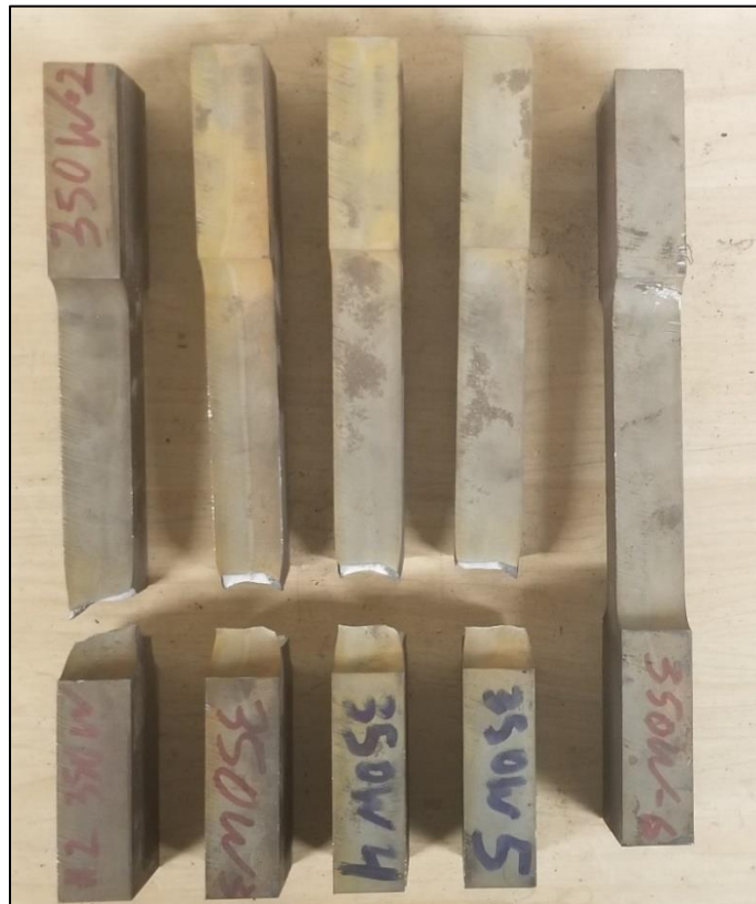
Figure 5-19: Side View of the Bare Coupons Made of 350W Post Fatigue
