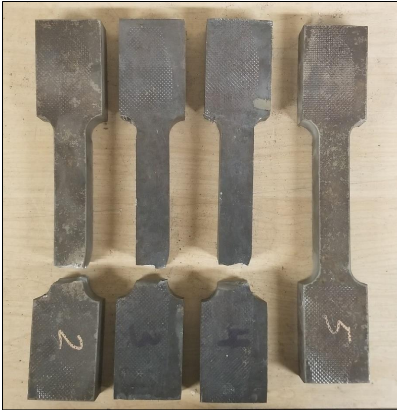
Figure 5-21: Top View of the Bare Coupons Made of A1010 Steel Post Fatigue
