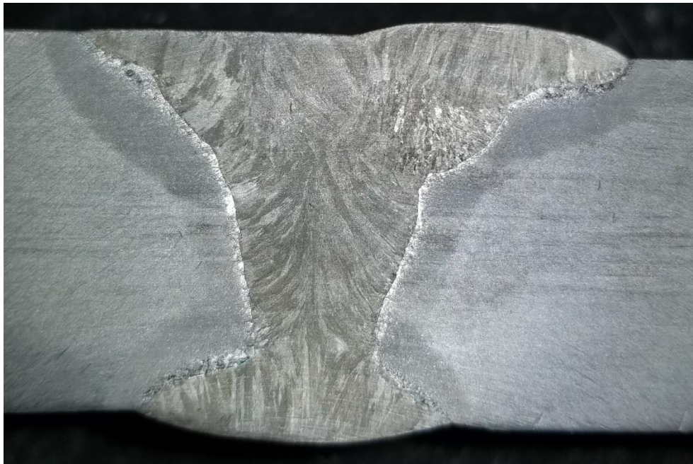
Figure 3-36: Close-Up View of Welded A1010 Specimen After Chemical Etching
