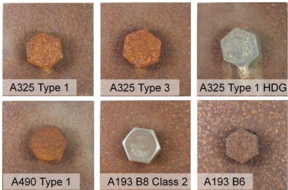
Figure 2-17: Galvanic Corrosion on Various Types of Fastener Systems Paired with A1010 plate (Groshek and Hebdon, 2018)
