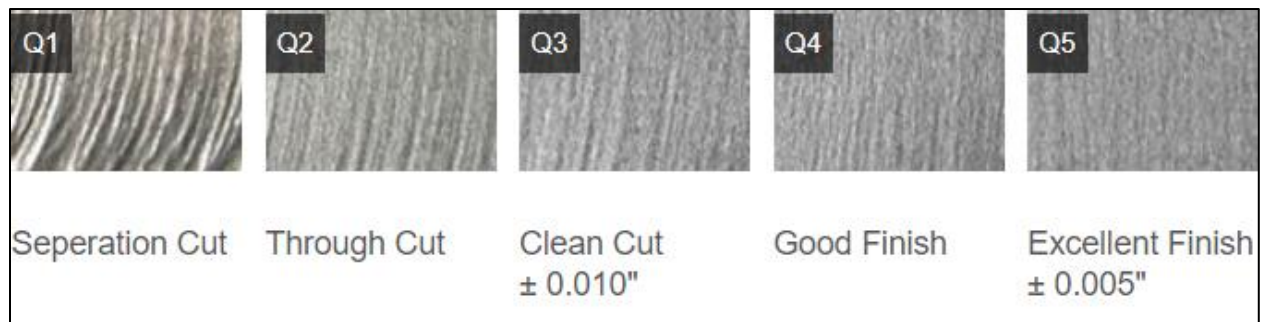
Figure 3-27: Difference in Waterjet Cutting Edge Quality (Source: WARDJet, wardjet.com)
