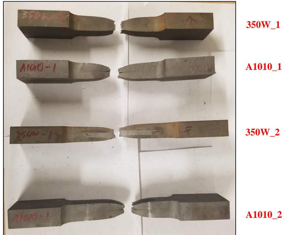
Figure 5-8: Side View of A1010 vs 350W Tensile Coupon Specimen Fracture
