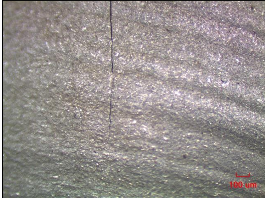
Figure 5-15: A1010 Delaminated Fracture Crack Tip and Discontinuities from Abrasive Cutting
