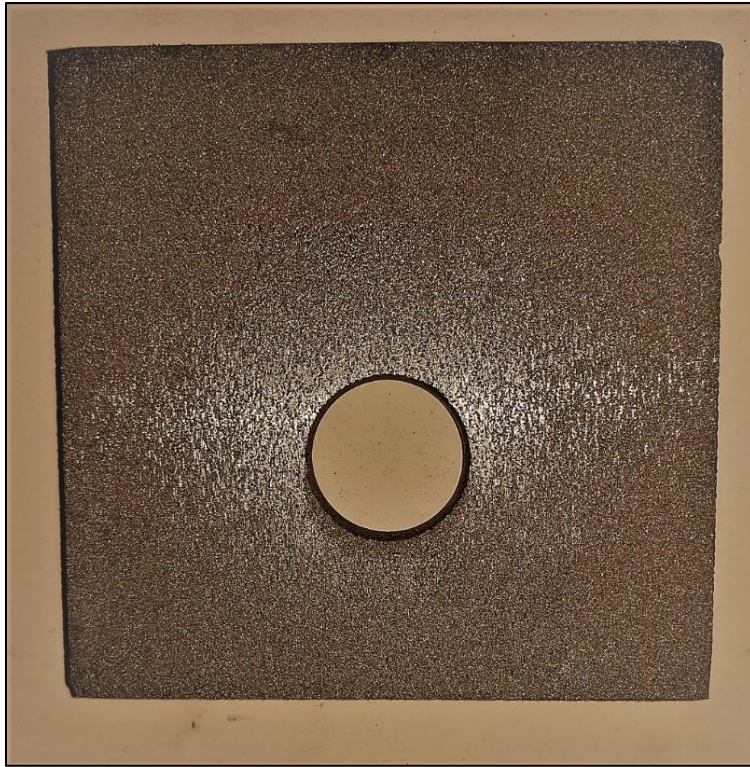
Figure 4-4: Filtered photo of A1010 plate showing slip area
