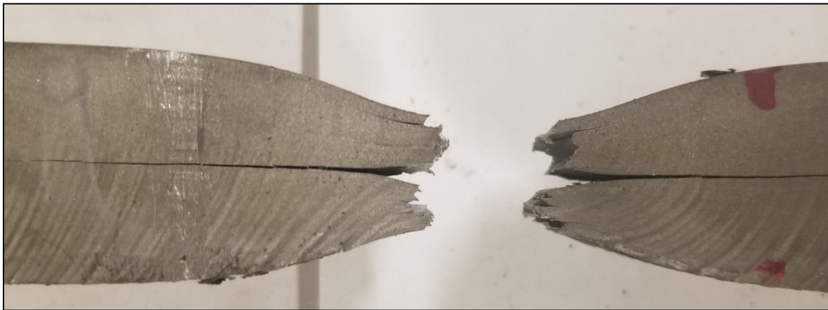
Figure 5-6: Close-Up View of A1010 Delaminated Fracture
