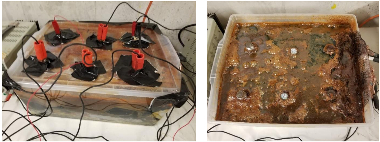
Figure 3-20: Accelerated Testing Setup Post-Corrosion
