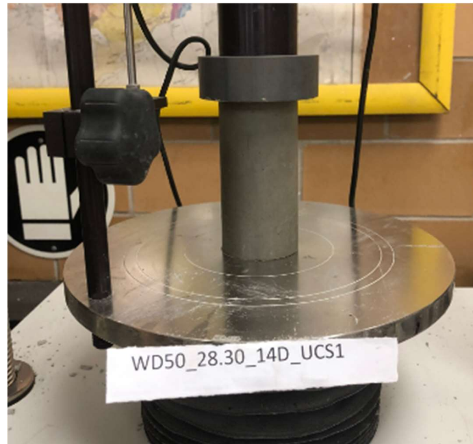
Figure 3-4: UCS Experimental Setup
