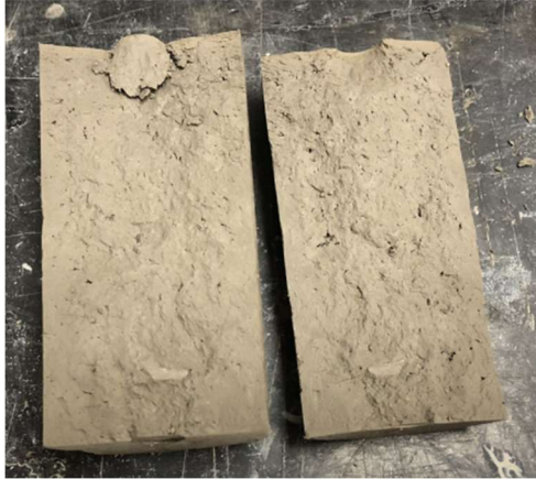
a) A proper split failure
