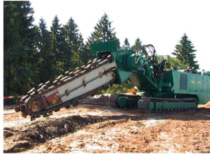
Figure 2-4: Trenching Machine Used in Horizontal Axis Deep Mixing (Massarsch & Topolnicki, 2005)
