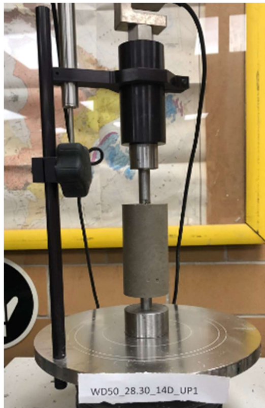
Figure 3-6: Typical UPT Setup
