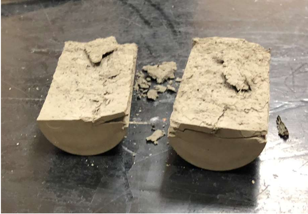
Figure 4-12: Failed Brazilian tensile specimen by splitting
