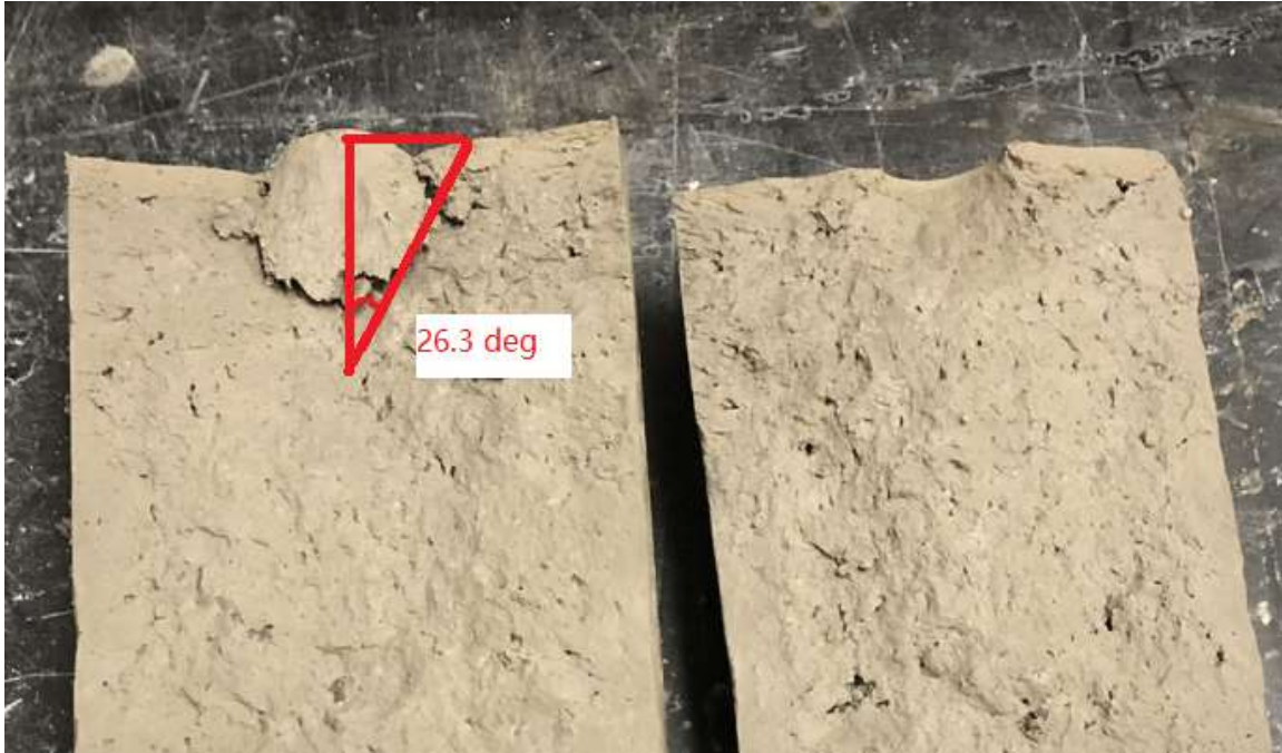
Figure 3-11: Angle \alpha Determination in UPT Specimens
