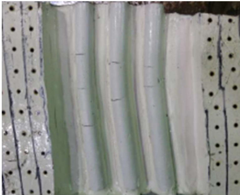
Figure 2-12: Physical Model of DSM Columns Under Loading. Certain Parts of the Columns Are Under Tension. (Nguyen et al., 2016)
