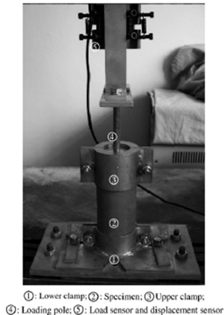
Figure 2-14: Direct Tensile Testing Setup (Wang et al., 2007)
