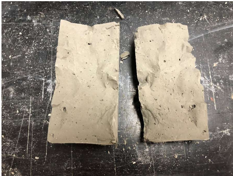
Figure 4-32: A Fractured Surface of Sample Tested with a 60° Penetration Disc
