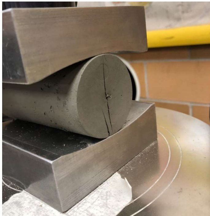
Figure 4-11: Failure and crack formation of a Brazilian tensile specimen
