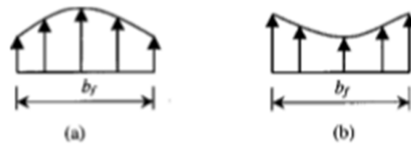
Figure 2.2. Stress profile across beam flange (a) strong-axis connection (b) weak-axis connection. Adapted from “Cyclic response and design recommendations of weak-axis reduced beam section moment connections” by C.S. Gilton and C. Uang, 2002, Journal of Structural Engineering Vol.128, Issue 4 . Copyright 2002 by the American Society of Civil Engineers.
