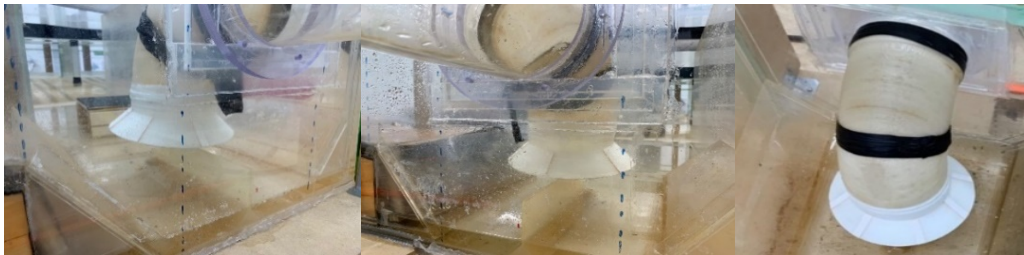
Figure 21. Tapered bell design installed on line A
