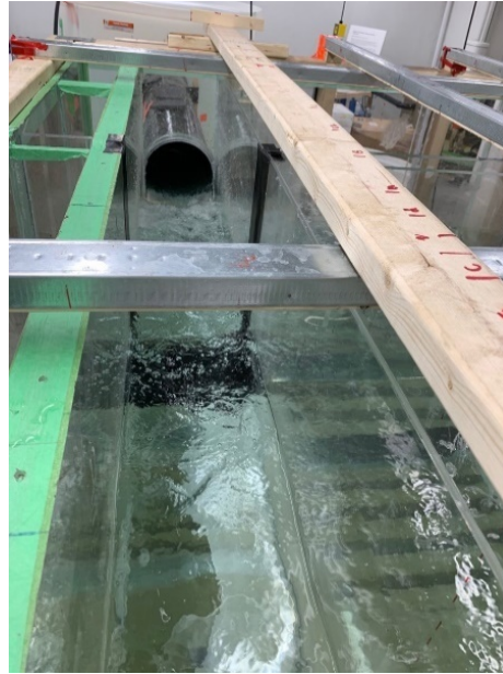
Figure 18. Inlet pipe flow conditions for the pump ABD combination with a flow 10 l/s for each pump by blocking 35% of Opening A and 45% of Opening B
