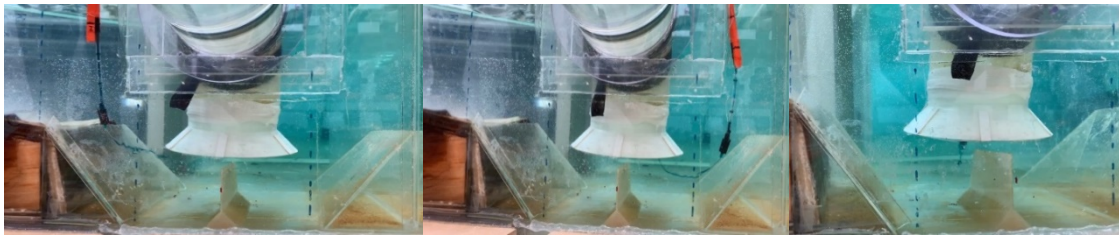
Figure 24. Dye injection at lateral and front sides of the tapered bell under cleaning cycle scenario
