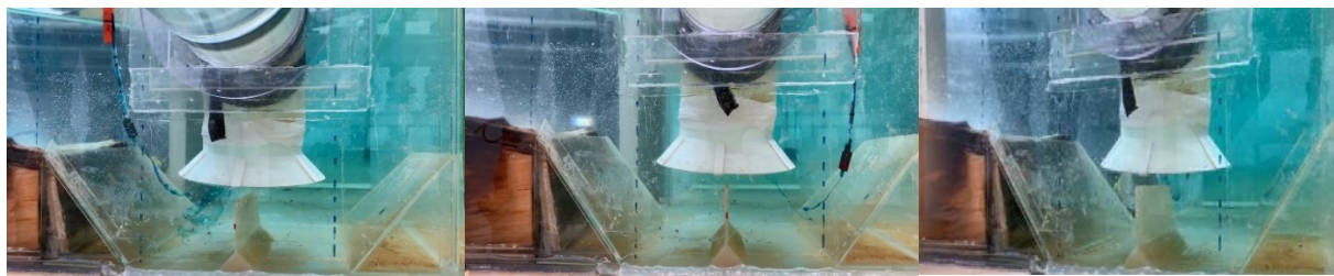
Figure 22. Dye injection at lateral and front sides of the tapered bell under low flow condition
