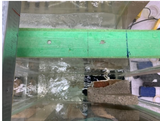
Figure 15. The 35% area of slot A was covered by foam sheet and bricks
