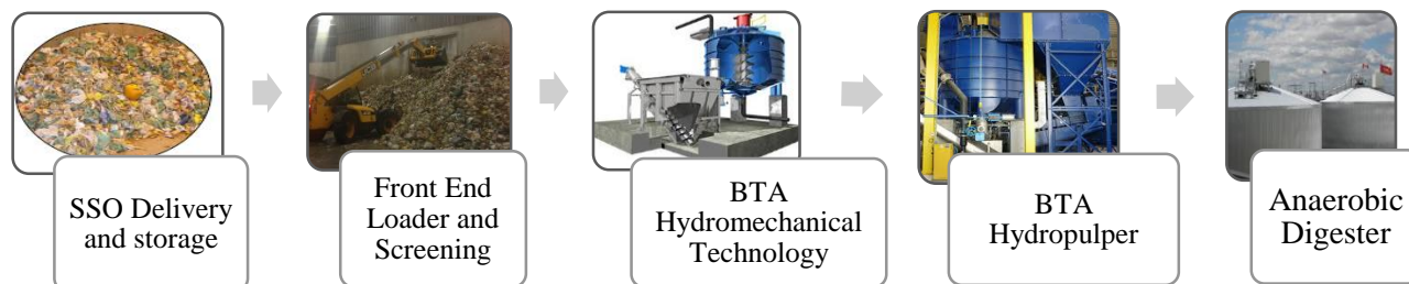
Figure 3.2. Source separated organics processing in Disco Road Facility
