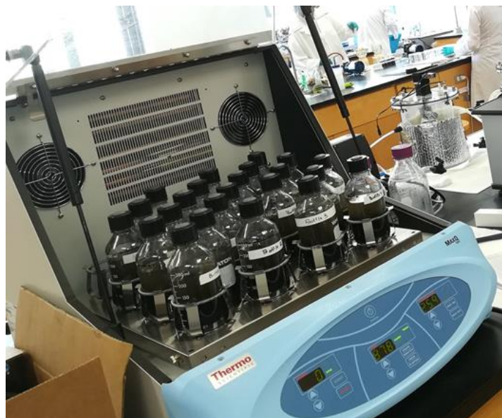
Figure 3.3- Experimental set-up for biomethane potential experiment
