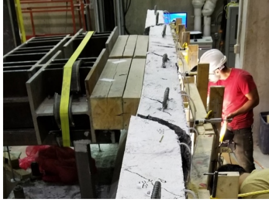
e) Punching shear failure pattern between the beginning and end of the loaded length
