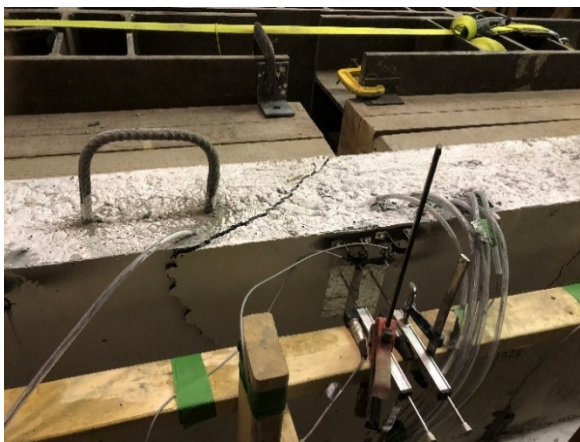
c) Local punching shear crack appeared in the gap between the two timber blocks of loading frame
