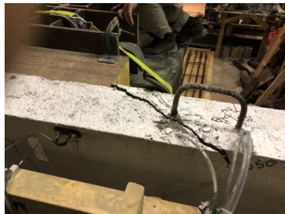
b) Punching shear crack appeared at the south end of the timber block of the loading frame
