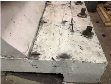
c) Flexural cracks in the cantilever end at south side
