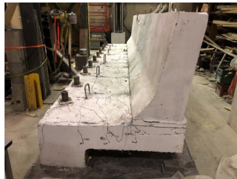
d) Flexural cracks in the cantilever end at the north side
