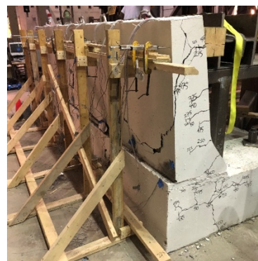
d) Propagation of the punching shear plane along the patch loading length
