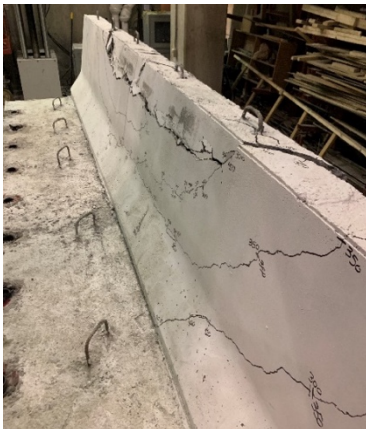
c) Side view of the punching shear failure
