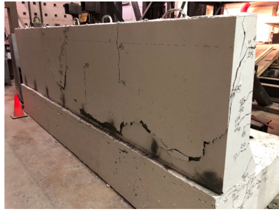
d) Propagation of the punching shear plane along the loaded length
