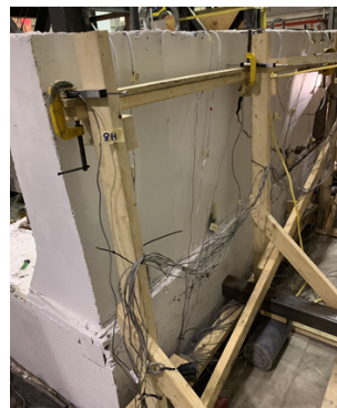
d) Punching shear crack at the north end of between the timber blocks in the loading frame loaded length that propagated to the south side of the loaded length
