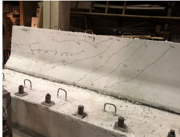
h) Front view of flexural cracks in the wall
