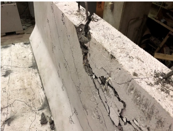
i) First punching shear crack to appear at the south end of the loaded length
