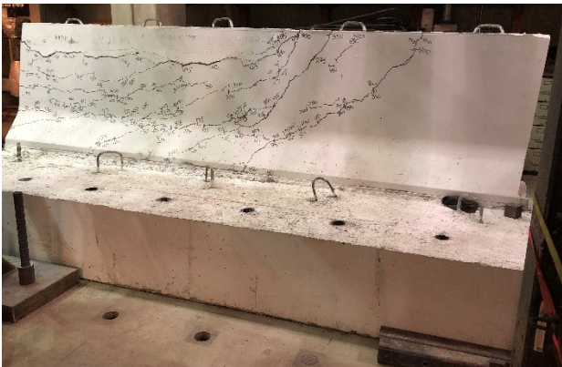
i) Crack pattern at failure
