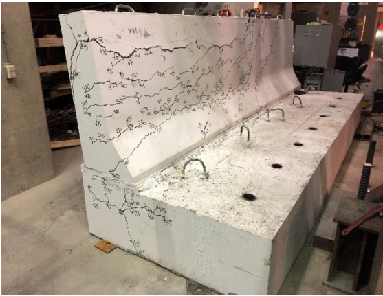
c) General view of final crack pattern
