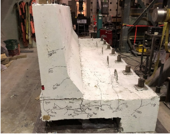
a) Flexural cracks in the barrier wall and deck at the south end
