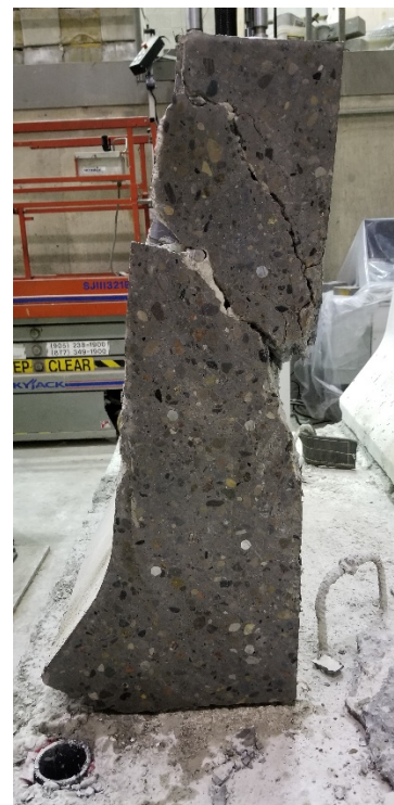
b) Saw cast at 100 mm away from the center of applied load towards the north end showing 40^\circ angle for the global punching shear crack while the local punching shear crack appeared on top of it in the right photo
