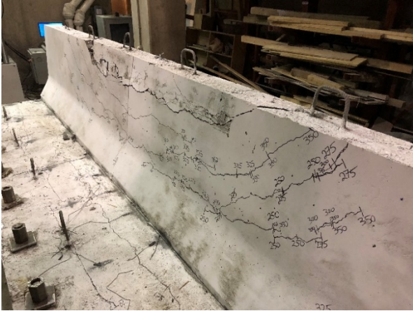
g) Looking south, horizontal cracks within the loaded length, in the tapered portion only, extending diagonally in the unloaded barrier portion
