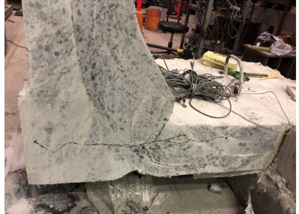
b) Saw cut at 1 m away from the center of barrier length in the unloaded portion, looking north, showing flexural crack in the deck and anchorage crack for embedded bent bar in deck
