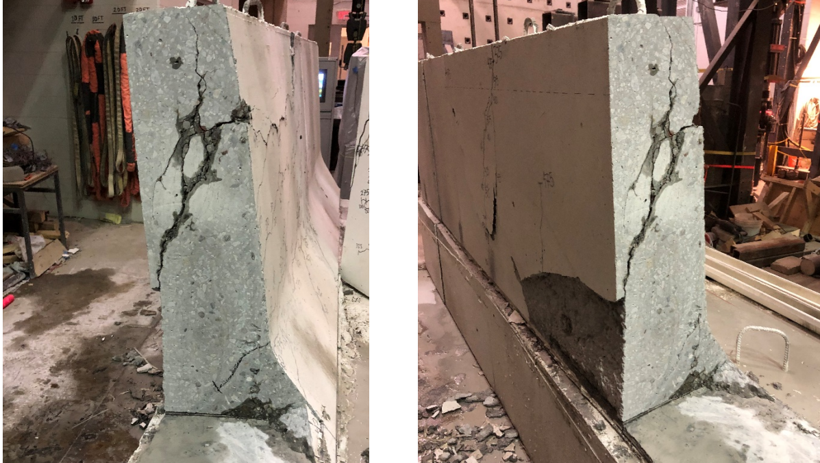
Figure 4.3 Saw cut at center of 1 m from the south end of barrier specimen S-1, looking north, showing 38° angle of punching shear failure
