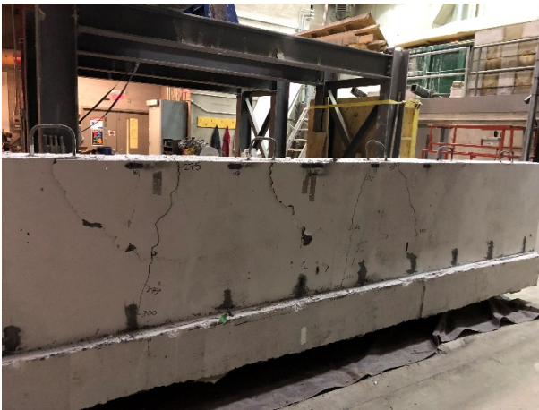
m) Slightly vertical cracks appeared within the loaded length close to failure load
