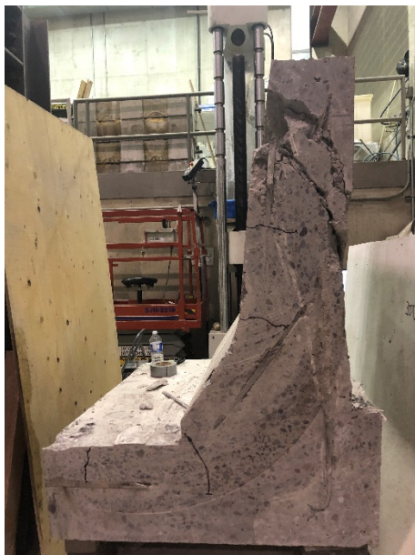
b) Saw cast at 100 mm away from the centre of applied load towards the north end showing 40° angle for the global punching shear crack while the local punching shear crack appeared on top of it in the left photo
