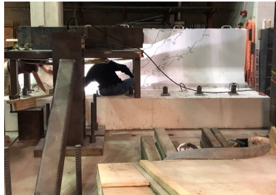
b) Propagation of horizontal cracks with the loaded length that propagated diagonally towards the unloaded barrier portion
