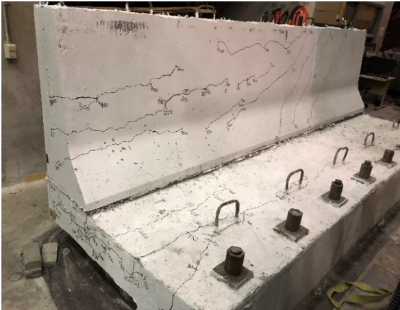
g) Flexural cracks in the barrier and deck viewed from the south side
