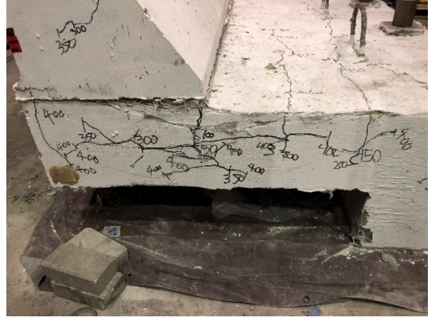
b) Close-up view of flexural cracks and bar anchorage crack in the deck cantilever
