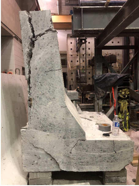
a) Saw cast at 1 m away from the centre of applied load towards the south end showing punching shear crack
