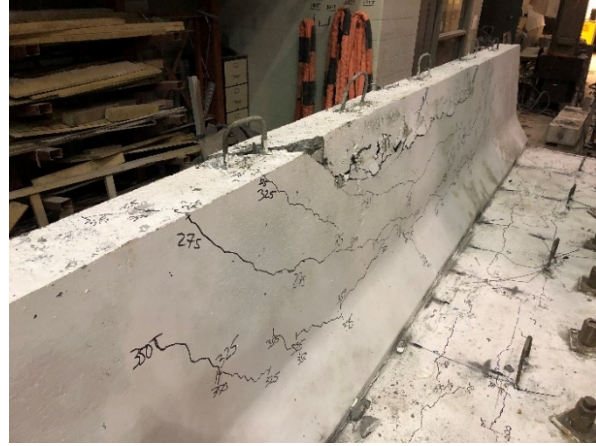
h) Looking north, horizontal cracks within the loaded length, in the tapered portion only, extending diagonally in the unloaded barrier portion
