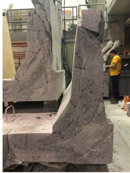
a) Saw cast at 1 m away from the centre of applied load towards the south end showing punching shear crack
