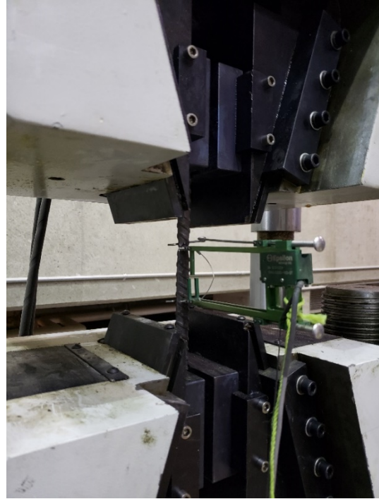
(c) Views of the test setup for 15M reinforcing steel coupon # 3 before testing (left) and after failure (right)
