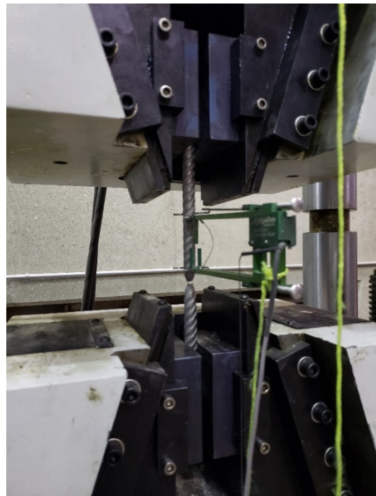
(e) Views of the test setup for 20M stainless steel coupon # 2 before testing (left) and after failure (right)
