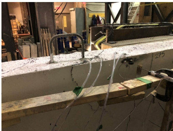
d) Punching shear crack appeared at the north end of the timber block of the loading frame
