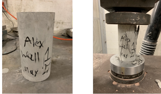
Figure 3. 3 A typical concrete cylinder before (left) and after (right) compression test
