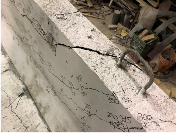
k) Second punching shear crack appeared at the north end of the loaded length when attempting to increase the applied load
