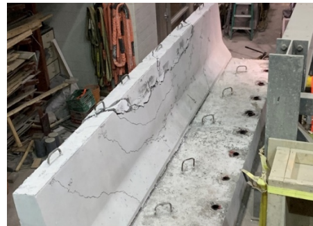
b) Pnching shear crack and flexural cracks extending diagonally in the unloaded portion, looking north
