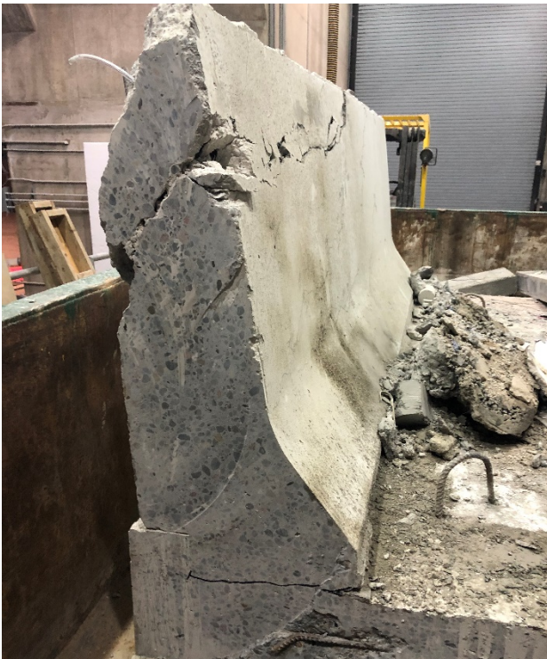
b) Saw cast at 100 mm away from the center of applied load towards the north end showing 40^\circ angle for the global punching shear crack while the local punching shear crack appeared on top of it in the right photo
