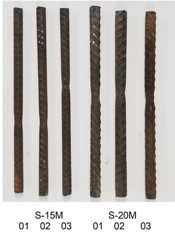
(g) Views of the failed reinforcing steel coupons
