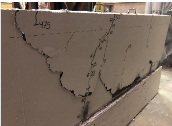
e) Punching shear at end of loaded length
