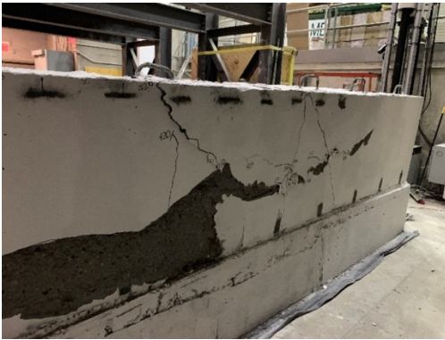
g) Local punching shear crack at top of wall between the timber blocks that did not propagate further
