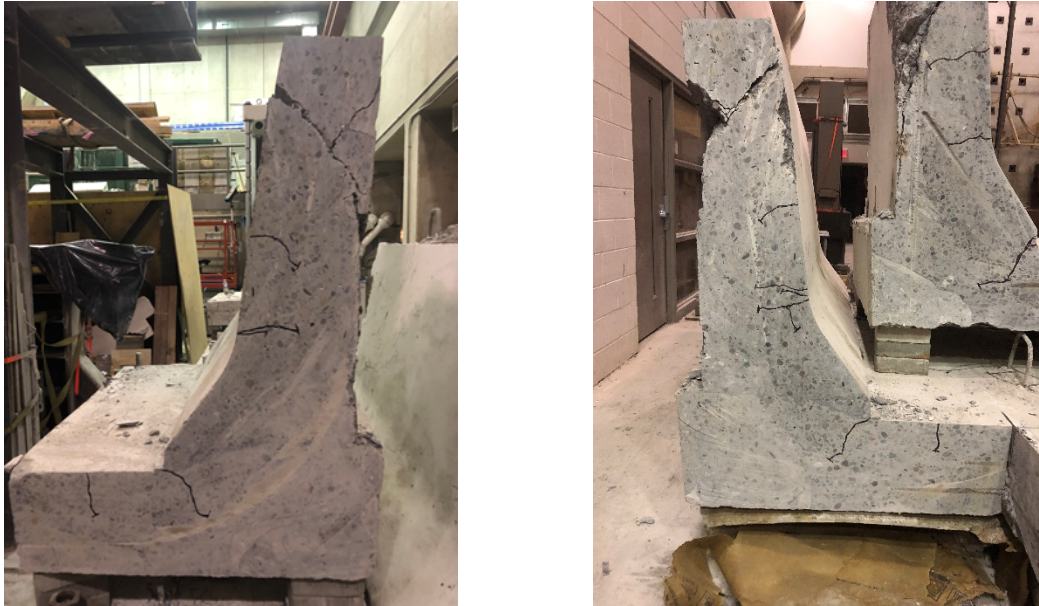
c) Saw cast at 1 m away from the centre of applied load towards the south end showing punching a 40^\circ punching shear crack
