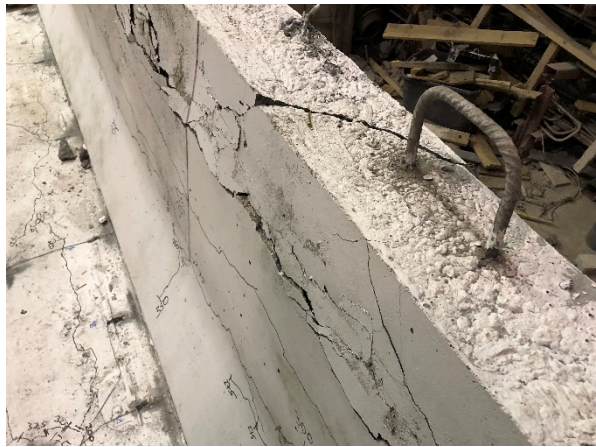
j) Local punching shear crack accompanied the first punching shear crack without extending further when attempting to increase the applied load
