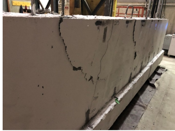
l) Punching shear cracks at beginning and end of the loaded length jointed together with signs of concrete popout when attempting to increase applied load
