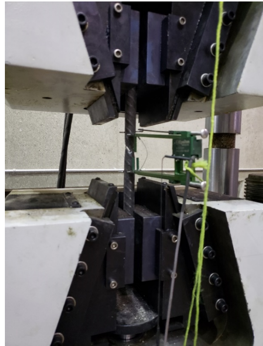
(d) Views of the test setup for 20M reinforcing steel coupon # 1 before testing (left) and after failure (right)
