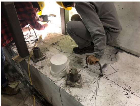
a) Recording flexural cracks in the deck slab cantilever during testing
