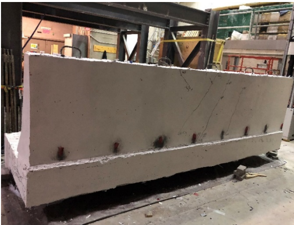
i) Crack pattern at back face of barrier showing slightly vertical cracks along the barrier loaded length
