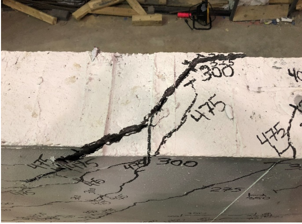
g) Top view of punching shear through barrier thickness
