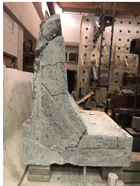
b) Saw cast at 100 mm away from the centre of applied load towards the north end showing 40° angle for the global punching shear crack while the local punching shear crack appeared on top of it in the left photo
