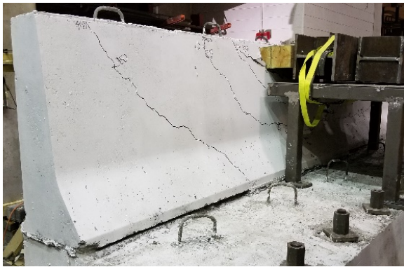
a) Horizontal cracks within the loaded length propagated diagonally in the unloaded portion of the barrier wall
