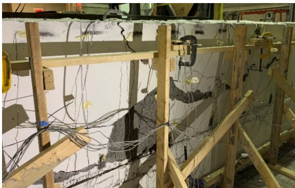
c) Local punching shear crack at top of wall that did not propagate further
