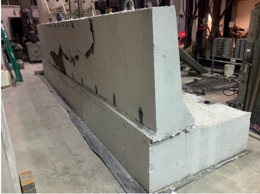
e) Punching shear failure at the south end of the loaded length
