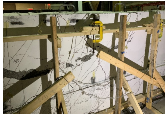
b) Punching shear crack at the south end of the loaded length that propagated to the north side of the loaded length
