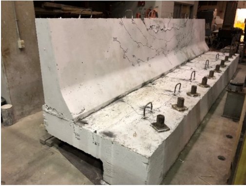
a) Crack pattern after failure, looking north
