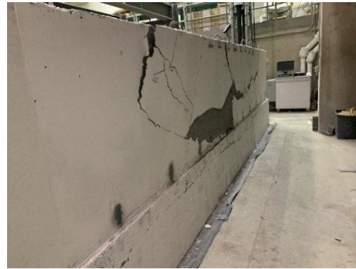
h) Punching shear crack at the north end of loaded length that propagated to the south side of the loaded length
