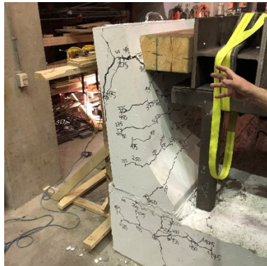
a) Flexural cracks in barrier wall and anchorage cracks in the concrete base
