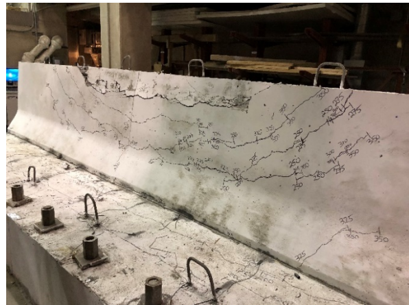
f) Flexural cracks extending all over the deck cantilever within and outside length
