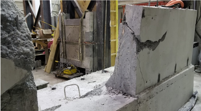
a) Saw cast at 1 m away from the center of applied load towards the south end showing 40^\circ angle for the punching shear crack
