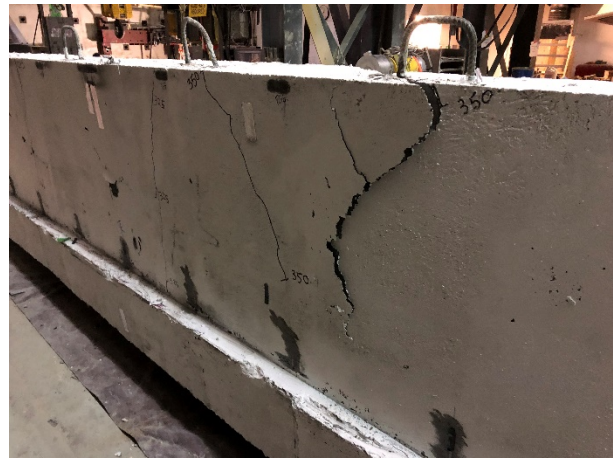
n) Punching shear crack at the south end of the loaded length
