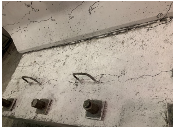
d) Propagation of flexural crack along the length of the deck cantilever
