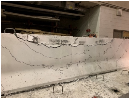
a) Front view of flexural cracks within the loaded length
