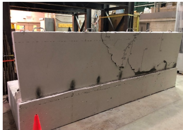
f) Vertical crack at back face at 1.8 m from the barrier's south end
