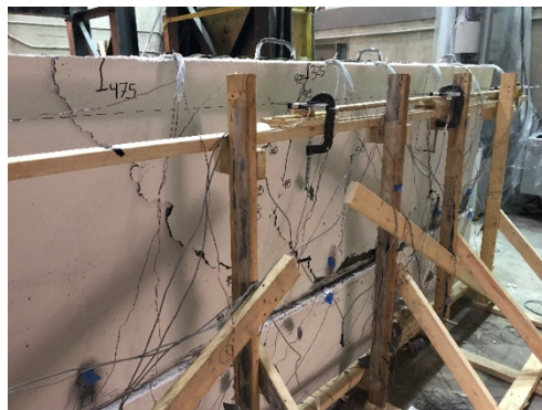
c) Punching shear crack at internal end of the patch loading
