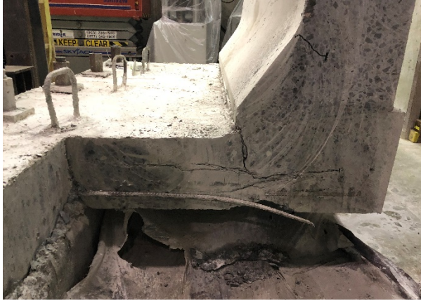
a) Saw cut at center of barrier length, looking south, showing flexural crack in the deck, anchorage crack for embedded bent bar in deck, and flexural crack at point of intersection of tapered portions in front side of barrier
