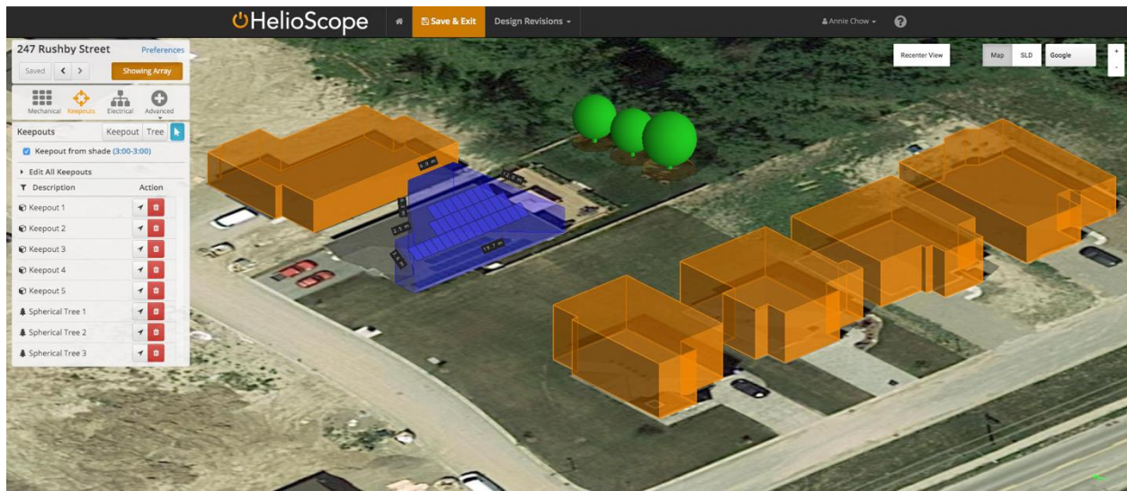
Figure 14. 3D view of case study area with neighbouring buildings and trees modeled as keepouts.
