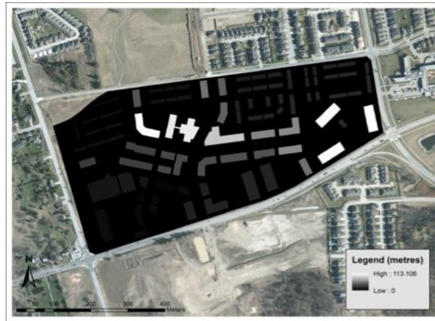
Figure 6. Original site plan design—converted 2D raster digital elevation model (DEM) at a resolution of 0.5 m converted from 3D file, projected onto orthophoto.
