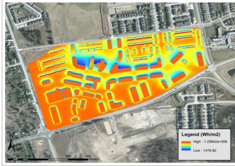
Figure 9. Example of an annual solar insolation map generated from the methodology for the original site plan.
