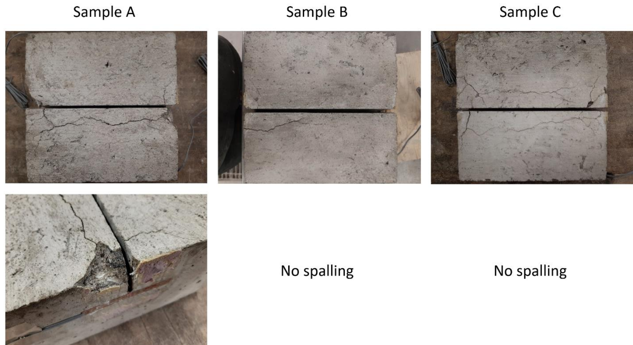
Fig. 8. Visual damage for 10% \text{CaCl}_2 under WD
