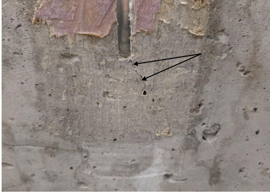
Fig. 5. Typical cracks developed in control samples under FT and FTW at the end of the 50 cycles
